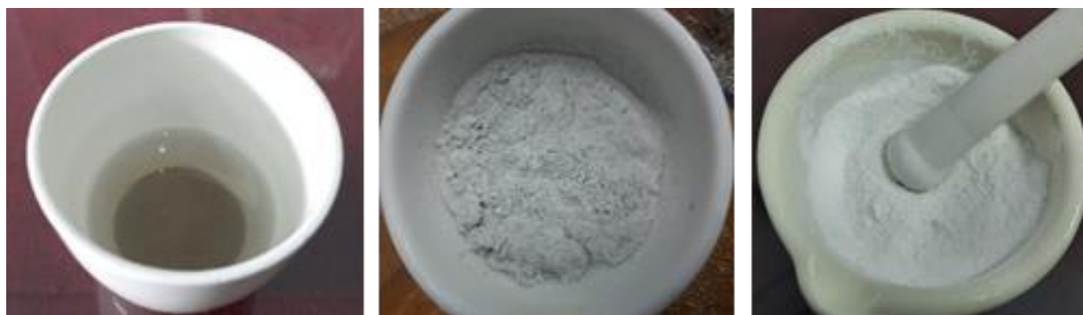
Figure 2. Preparation of silica powder by alkali-fusion reduction of sand.
