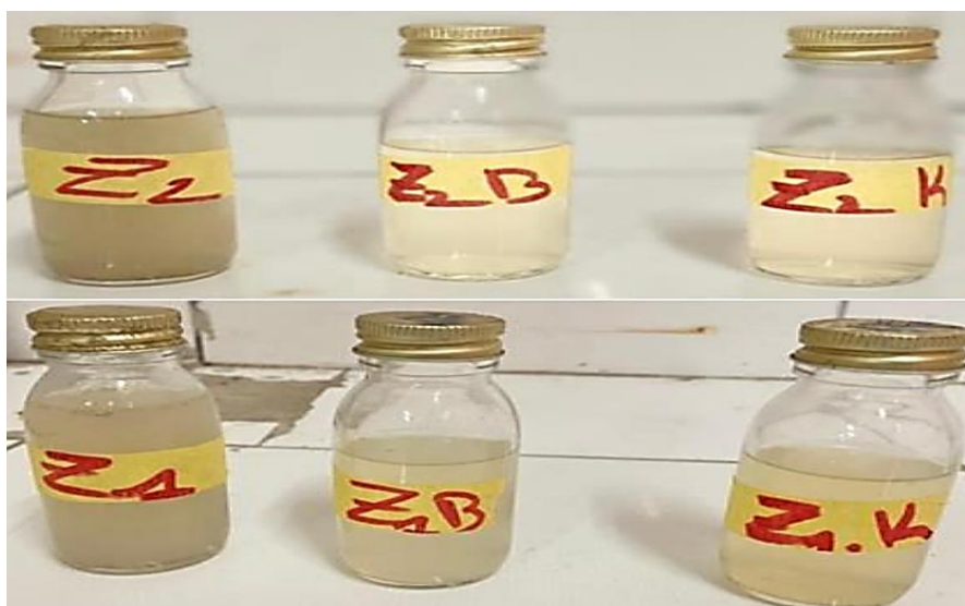
Figure 6. Industrial effluent samples before ( Z_1 and Z_2 ) and after clay treatment ( Z_{1\text{BIN}} ; Z_{1\text{KAT}} ; Z_{2\text{BIN}} and Z_{2\text{KAT}} )
