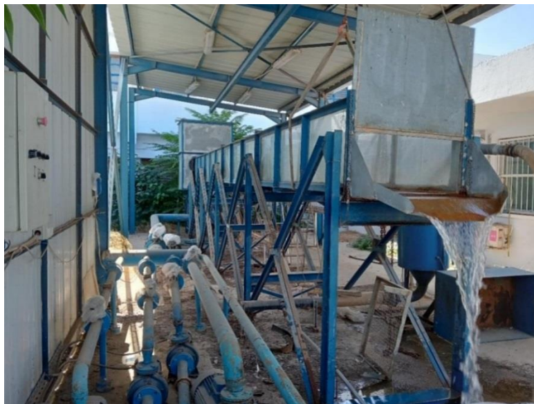
Figure 1. The INAT experimental channel (Length: 10m; width: 0.8m; height: 0.6m)
