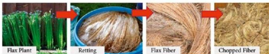
Figure 1. Extraction of flax fibers.
