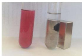
**Figure 1.** Illustration of BR46 removal by synthesized RGO/Fe<sub>3</sub>O<sub>4</sub> nanocomposites and their separation from the solution by magnet.
