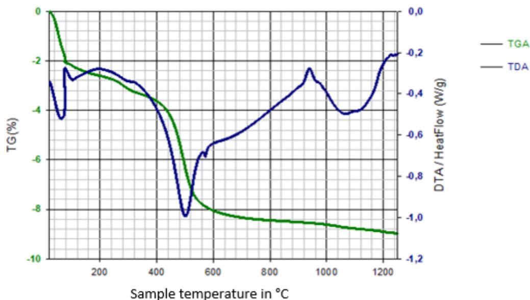
**Figure 1.** TGA/DTA curves of sample S1.
