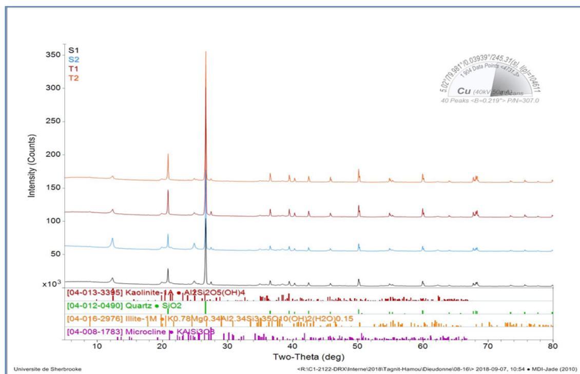
**Figure 5.** XRD spectra of raw clays of S1, S2, T1 and T2**Table 6.** Quantitative Mineralogical Compositions of Samples S1, S2, T1 and T2.
