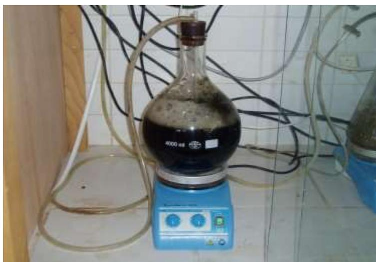
**Photo 1.** Aerobic process for leachate treatment
