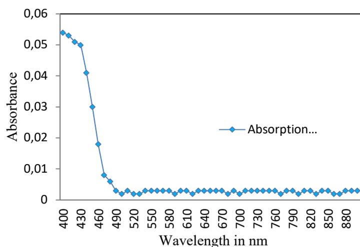
**Figure 3.** Absorption spectra of MAP
