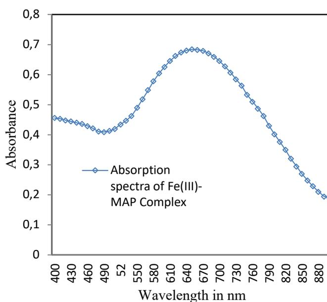
**Figure 4.** Absorption spectra of [Fe(III) - MAP] complex for  $50 \mu\text{g cm}^{-3}$  of Fe(III)
