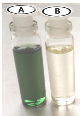
**Figure 1.** A) Color Response of MAP with  $Fe^{+3}$  ions in alcoholic medium at ambient temperature. B) Color Response of MAP in absence of  $Fe^{+3}$  ions in alcoholic medium at ambient temperature (Blank).
