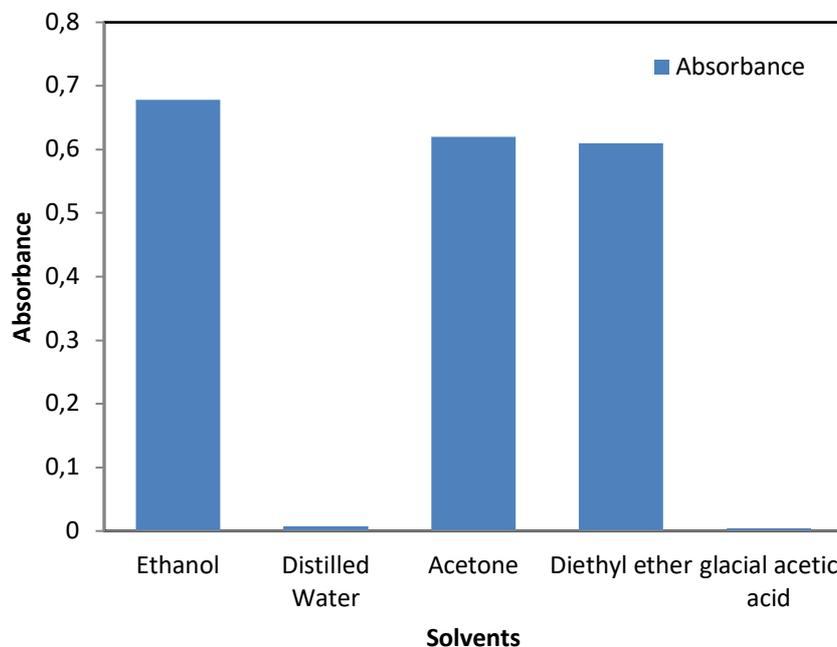
**Figure 5.** Effect of different solvents on [Fe(III) - MAP] complex formation
