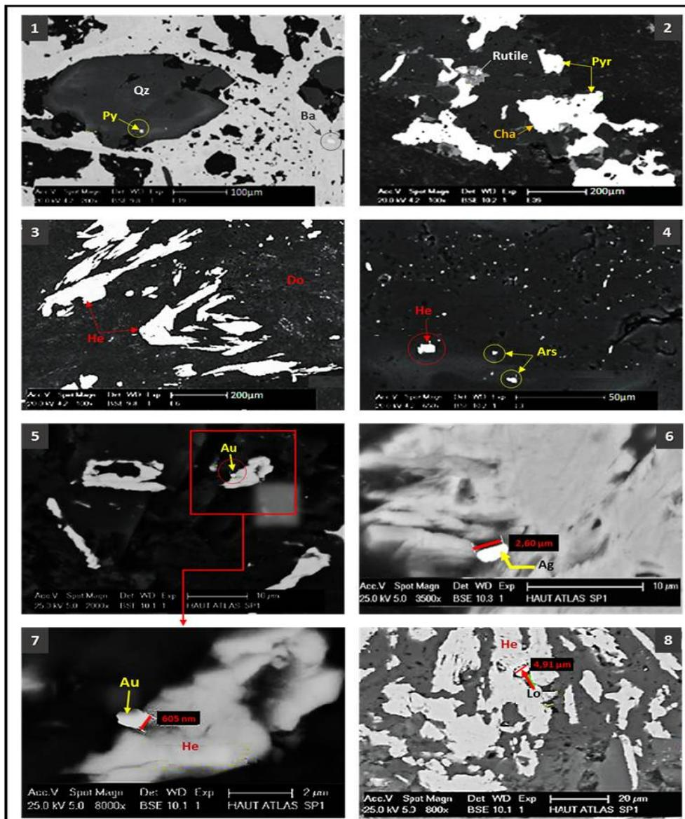
**Figure 5 :** SEM Photomicrographs showing: (1) Quartz with pyrite inclusion (2) Chalcopyrite associated with pyrrhotite (3) Iron oxide (4) Quartz with arsenopyrite inclusions (5) - (6) Golden grain. (7) Silver grain (8) Lollingite.
