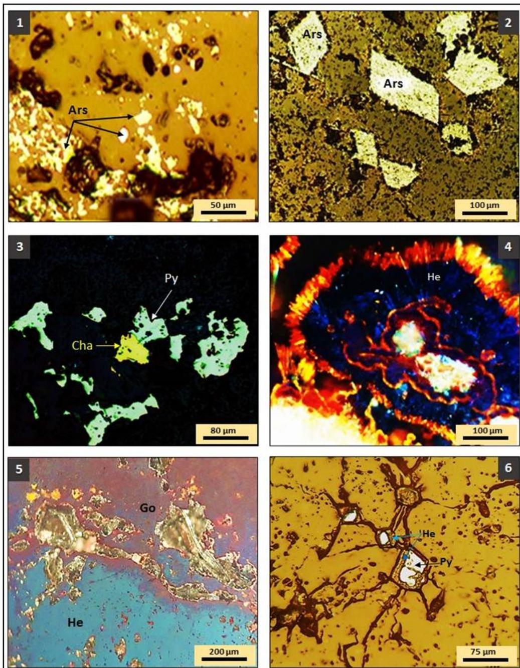
**Figure 4:** Photomicrographs in reflect light of Albour ores: (1) carried texture of arsenopyrite. (2) Automorphic Arsenopyrites (3) Chalcopyrite associated with pyrrhotite. (4) Botryoidal texture of acicular hematite. (5) Hematite-goethite association. (6) Pyrite pseudomorphosed by hematite.
