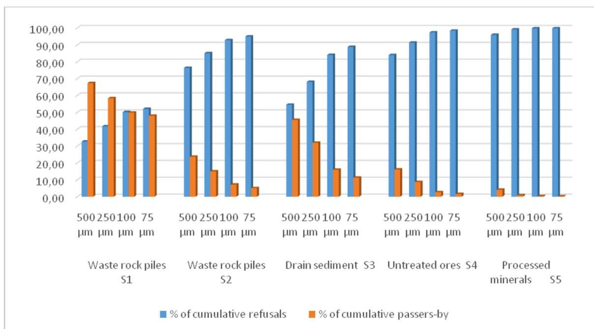
Figure 3: Particles size distribution in the residue
