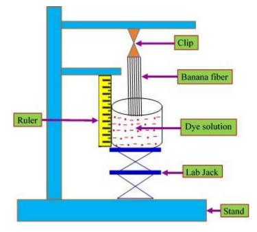
Figure 2 Schematic illustration of the experimental setup of wicking test of banana fiber.
