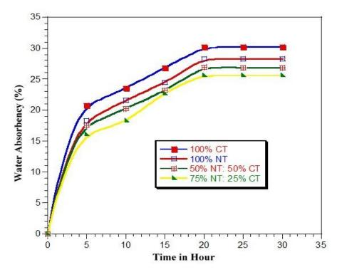
Figure 5 Plots of water absorption vs time of 100%CT, 100%NT, 75NT:25CT and 50NT:50CT
