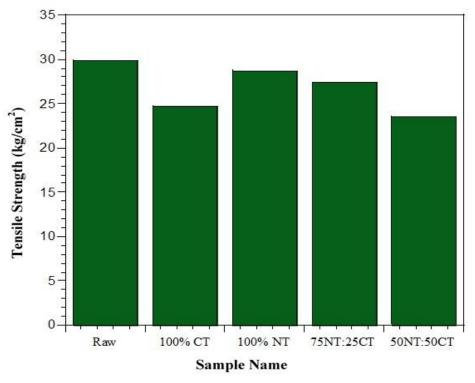
Figure 7 Tensile behavior of Raw, 100% CT, 100% NT, 75NT:25CT and 50NT:50CT banana fibers.
