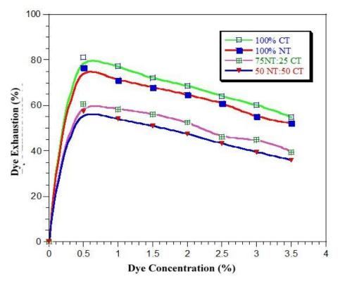
**Figure 6** Plots of dye exhaustion vs dye concentration for 100%CT, 100%NT, 75NT:25CT and 50NT:50CT banana fiber.
