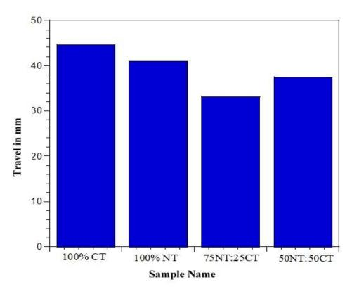
Figure 4 Wicking properties of 100% CT, 100% NT, 75NT:25CT, and 50NT:50CT banana fiber.
