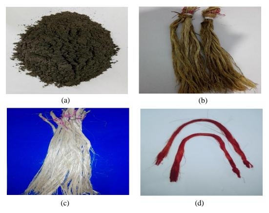
**Figure 1** Photographs of (a) Banana tree trunk ash (b) Scoured banana fiber (c) Bleached banana fiber and (d) Dyed banana fiber.
