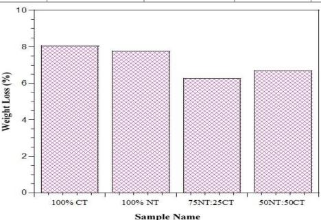
Figure 3 The percentage of weight loss of 100% CT, 100% NT, 75NT:25CT, and 50NT:50CT banana fiber.
