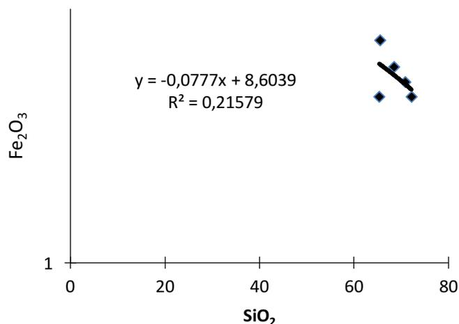
**Figure 6.** Variation of iron and alumina in function of silica on the Kaele's lithomorphic Vertisols
