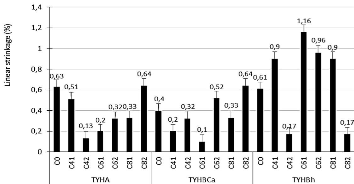
Figure 12. Linear shrinkage of stabilized specimens.
