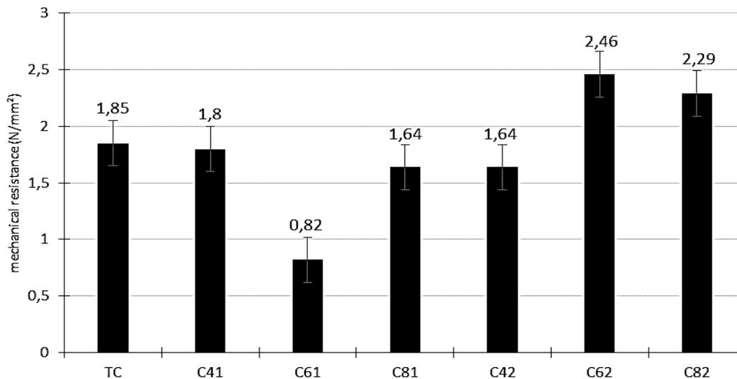
**Figure 15.** Mechanical resistance of specimens in function of lime concentration. TC = specimens of crude brick, C4, C6, C8 = concentration of lime (4, 6 and 8%); 1 and 2 design horizons.
