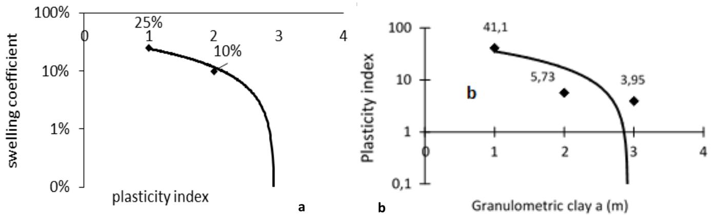
**Figure 10.** Swelling coefficient (a) and plasticity index (b) of Vertisols samples from the Tipili Yewey profile.
