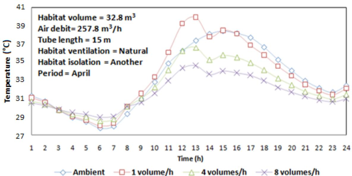
**Figure 9.** Evolution of the air temperature in the habitat for different renewal rates
