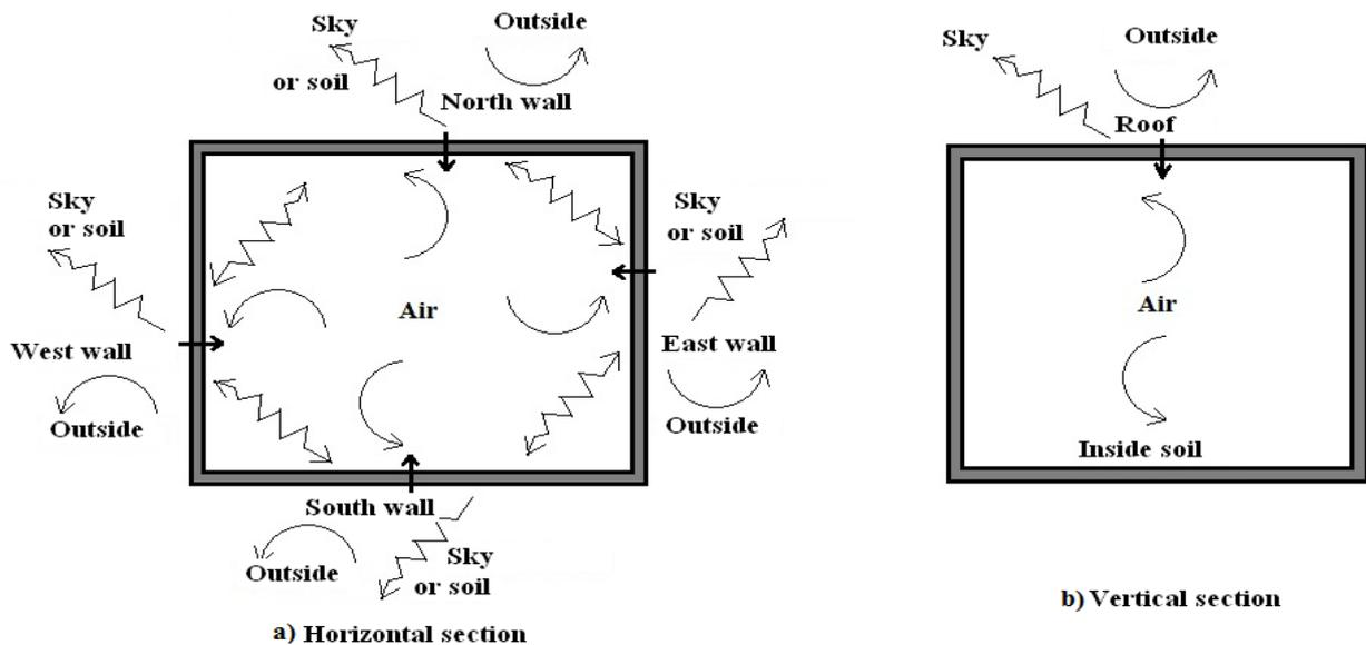
**Figure 3.** Scheme of thermal exchanges in the habitat.
