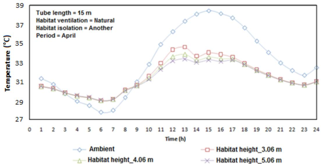
**Figure 10.** Evolution of the air temperature in habitat for different heights of the wall
