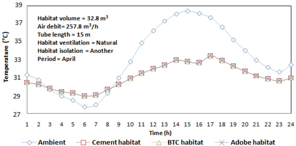
**Figure 7.** Evolution of air temperature in different types of habitat with insulated roof
