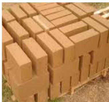
**Figure 2b.**The compressed earth block (BTC)
