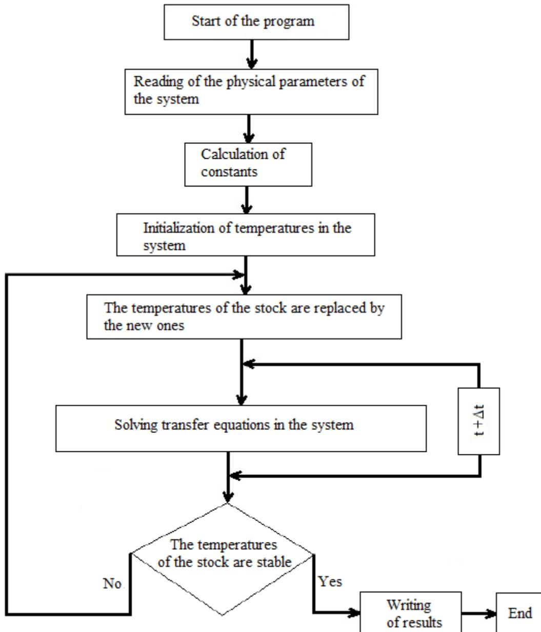
Figure 4. Algorithm of simulation program
