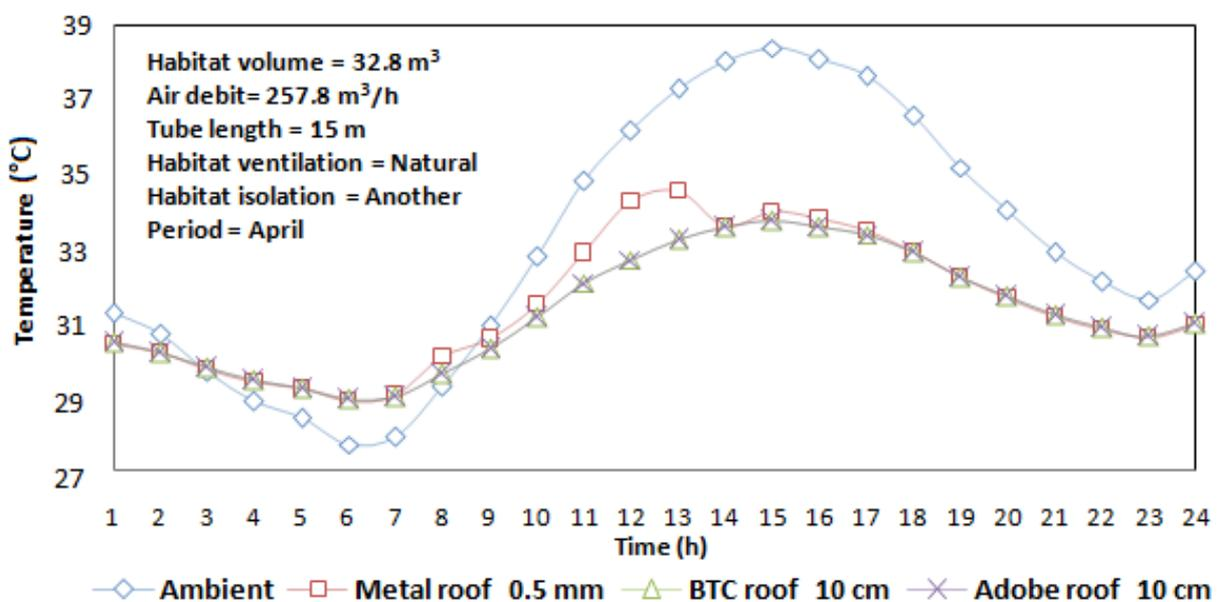
**Figure 8.** Evolution of the air temperature in habitat for different roofs
