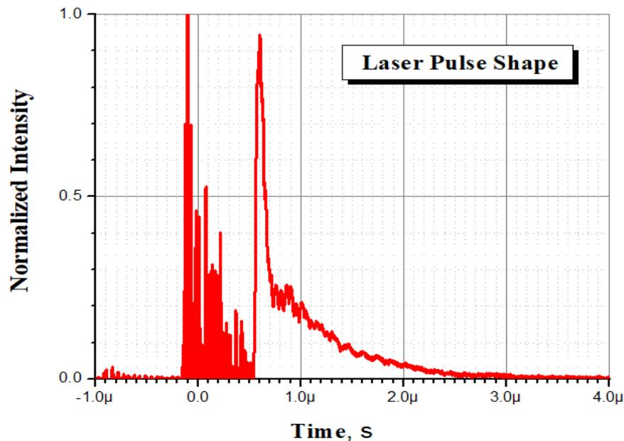
**Figure 9.** Laser Pulse Temporal Shape
