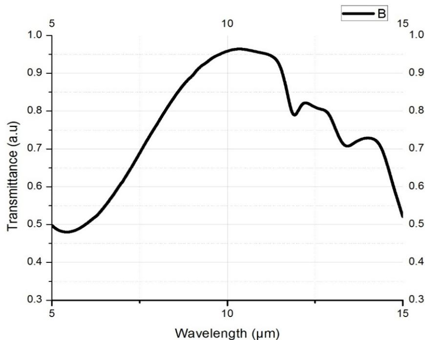
**Figure 3.** Transmittance versus wavelength for two side's anti-reflecting coated germanium sample
