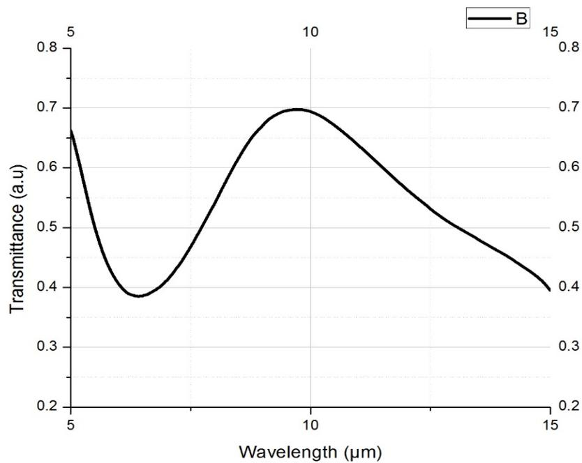
**Figure 5.** Transmittance versus wavelength for ZnSe coated by germanium with 1500 nm thickness
