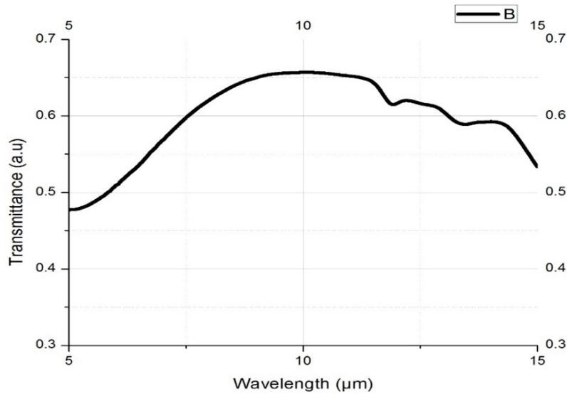
**Figure 2.** Transmittance versus wavelength for one side anti-reflecting coated germanium sample
