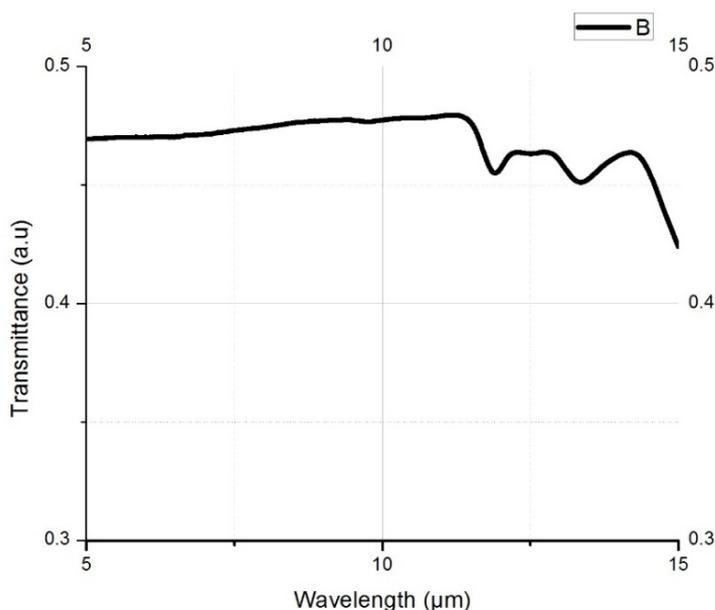
**Figure 1.** Transmittance versus wavelength for uncoated germanium sample
