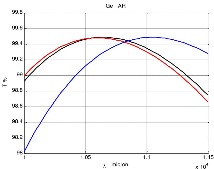
**Figure 6.** A comparison of the three coated layers. The red curve presents a quarter of wavelength of ZnS on germanium sample, the black curve represents the coating of 0.2405 optical thickness of ZnS wavelength with two layers of  $Y_2O_3$  having 0.005 optical thickness, while the blue curve represents the coating of quarter of ZnS wavelength with two layers of  $Y_2O_3$  having 0.005 optical thickness
