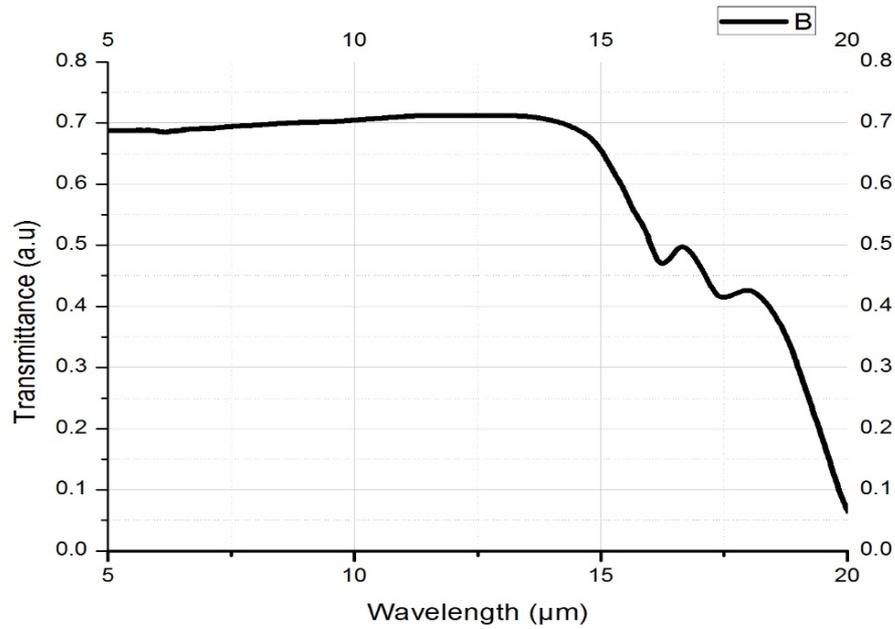
**Figure 4.** Transmittance versus wavelength for ZnSe without coating process
