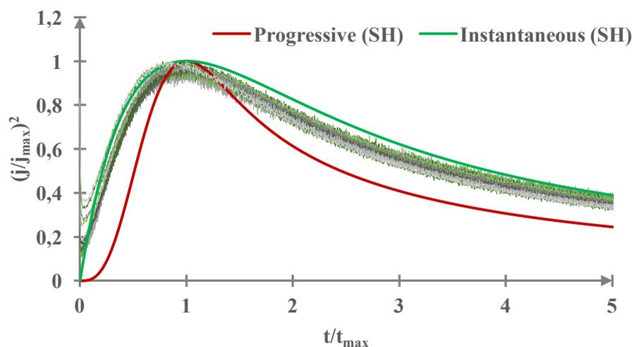
**Figure 6.** Non-dimensional plot of the current density transients for Cu deposition from 30 mmol of  $\text{Cu}(\text{NO}_3)_2 \cdot 3\text{H}_2\text{O}$  in ChCl-Ox at  $T = 70^\circ\text{C}$ .
