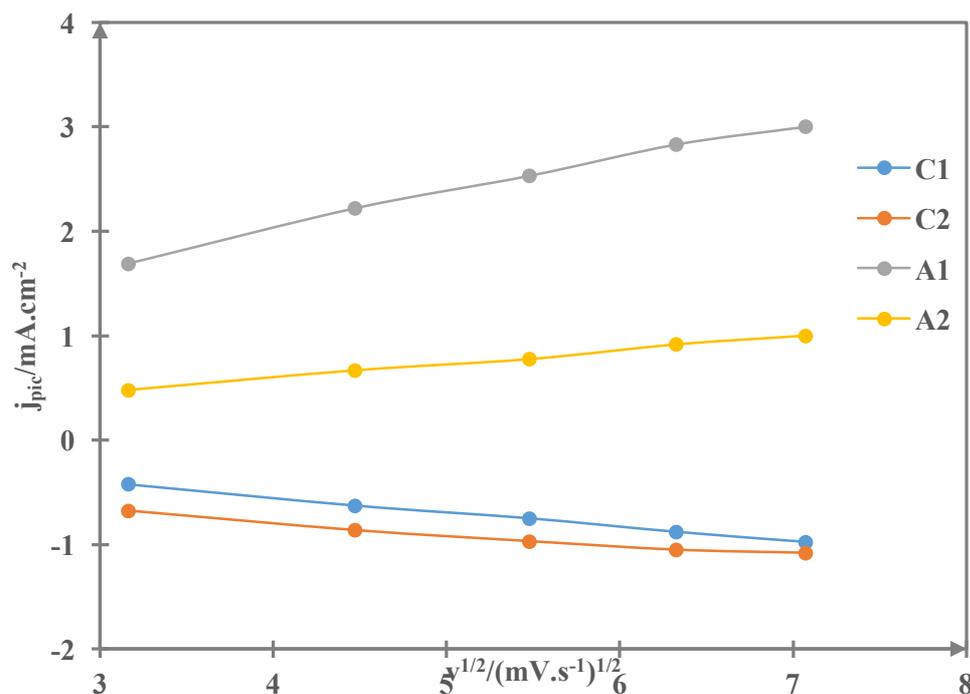
**Figure 4.** Current density at the peaks C1, C2, A1 and A2 vs square root of the scan rate ( $j_{peak} = f(v^{1/2})$ ) of ChCl-Ox with 30 mmolal of  $\text{Cu}(\text{NO}_3)_2 \cdot 3\text{H}_2\text{O}$  at GC electrode recorded at different,  $T = 70^\circ\text{C}$ .
