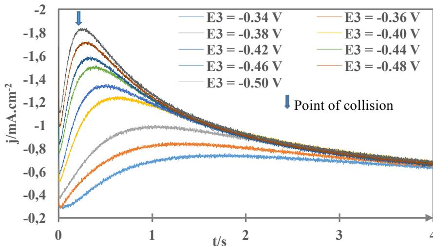
**Figure 5.** Experimental current density transients recorded from ChCl-Ox with 30 mmol of  $\text{Cu}(\text{NO}_3)_2 \cdot 3\text{H}_2\text{O}$  at GC after a potential step from -0.3 V to various final potentials indicated in the legend.  $T = 70^\circ\text{C}$ .
