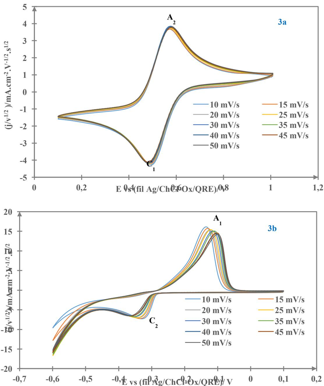
**Figure 3. (3a)** Current density normalized with respect to the square root of the scan rate ( $\frac{j}{v^{1/2}} = f(E)$ ) vs potential between potential range of 0.1 V and 1 V. Current density from cyclic voltammograms (3rd scan, figure 1) of ChCl-Ox with 30 mmolal of  $\text{Cu}(\text{NO}_3)_2 \cdot 3\text{H}_2\text{O}$  at GC electrode recorded at different scan rate and  $T = 70^\circ\text{C}$ .
