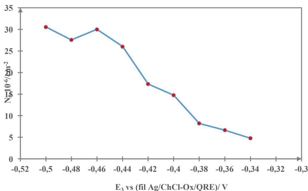
**Figure 7.** Evolution of the nuclei density vs the reduction potential of copper (I) to copper (0) in ChCl-Ox with 30 mmolal of  $\text{Cu}(\text{NO}_3)_2 \cdot 3\text{H}_2\text{O}$  at GC electrode,  $T = 70^\circ\text{C}$ .
