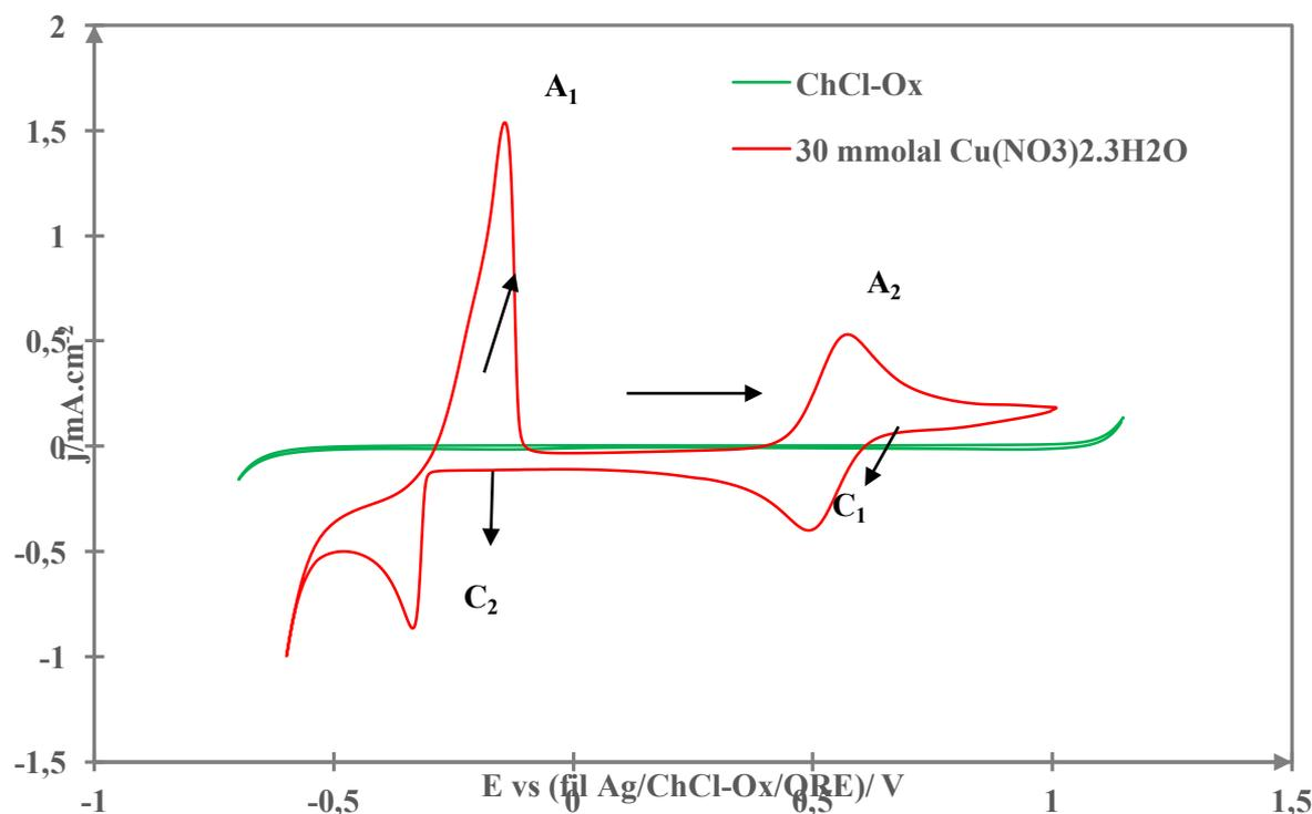
**Figure 1.** Cyclic voltammograms (3rd scan) of ChCl-Ox (green curve) and ChCl-Ox with 30 mmolal of  $\text{Cu}(\text{NO}_3)_2 \cdot 3\text{H}_2\text{O}$  (red curve) at GC electrode;  $v = 10 \text{ mV/s}$  and  $T = 70^\circ\text{C}$ .
