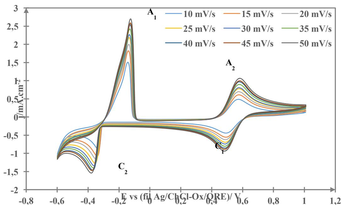
**Figure 2.** Cyclic voltammograms (3rd scan) of ChCl-Ox with 30 mmolal of  $\text{Cu}(\text{NO}_3)_2 \cdot 3\text{H}_2\text{O}$  at GC electrode recorded at different scan rate and  $T= 70^\circ\text{C}$ .
