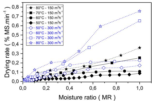
**Figure 2:** Variation of moisture ratio as a function of time. **Figure 3:** Variation of drying rate as a function of moisture ratio
