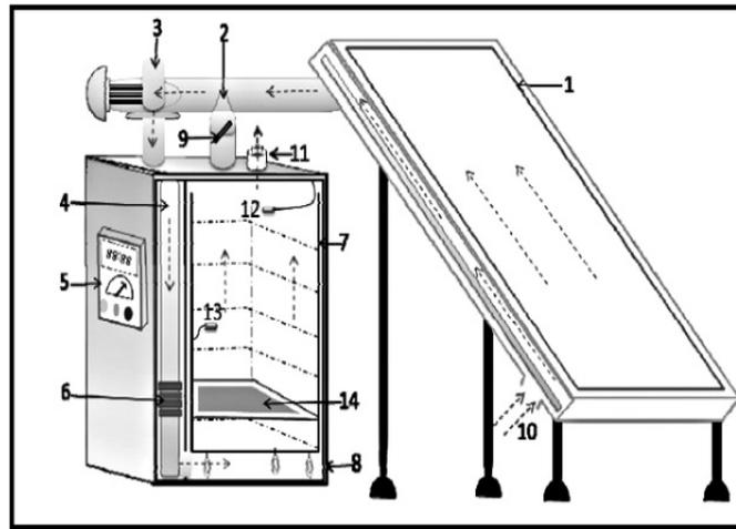
**Figure 1:** Schematic representation of the solar dryer : (1) solar collector; (2) circulation fan; (3) fan; (4) airflow direction, (5) control box; (6) auxiliary heating system; (7) shelves; (8) drying cabinet; (9) recycling air; (10) control foot; (11) exit of air; (12) humidity probes; (13) thermocouples.
