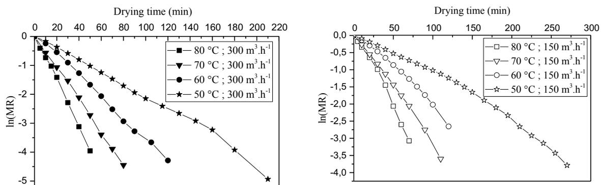
**Figure 5:** The effects of temperature and airflow on the effective diffusion coefficient of dandelion leaves
