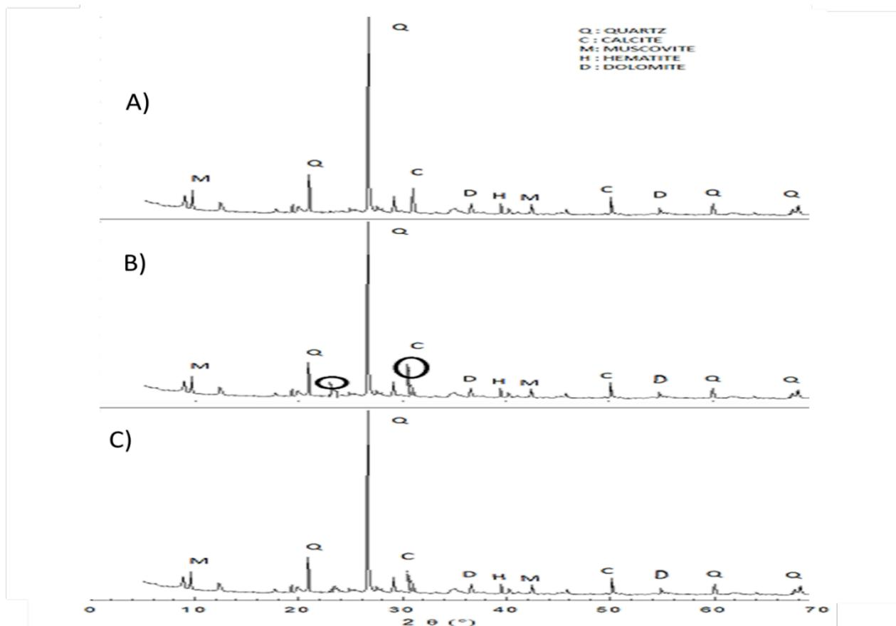
**Fig. 1.** The XRD pattern of the clay before adsorption (A), After adsorption (B), After regeneration (C)
