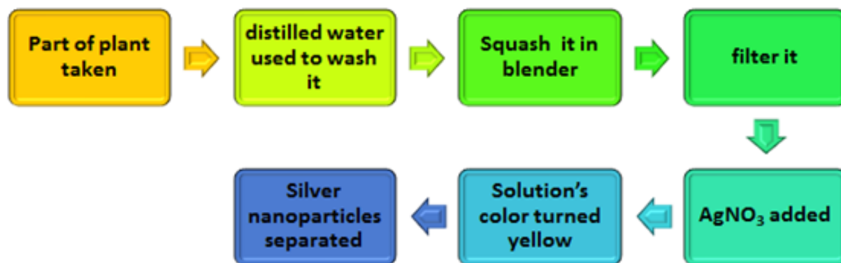
Figure 4: Process of in vitro synthesis of silver nanoparticles from different parts of the plant
