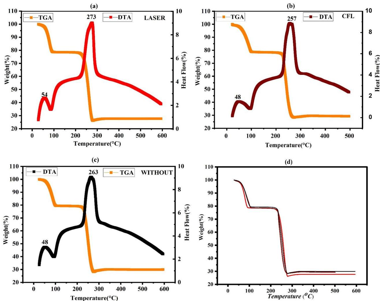
**Figure 5.** TGA/DTA plots of MgCT Crystals (a) Laser, (b) CFL, (c) without radiations, and (d) The overall changes in different conditions.
