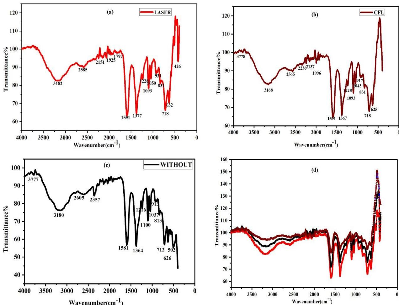
**Figure 4.** FTIR spectra of MgCT Crystals at (a) Laser, (b) CFL, (c) without radiation. And (d) The overall Changes in functional group.
