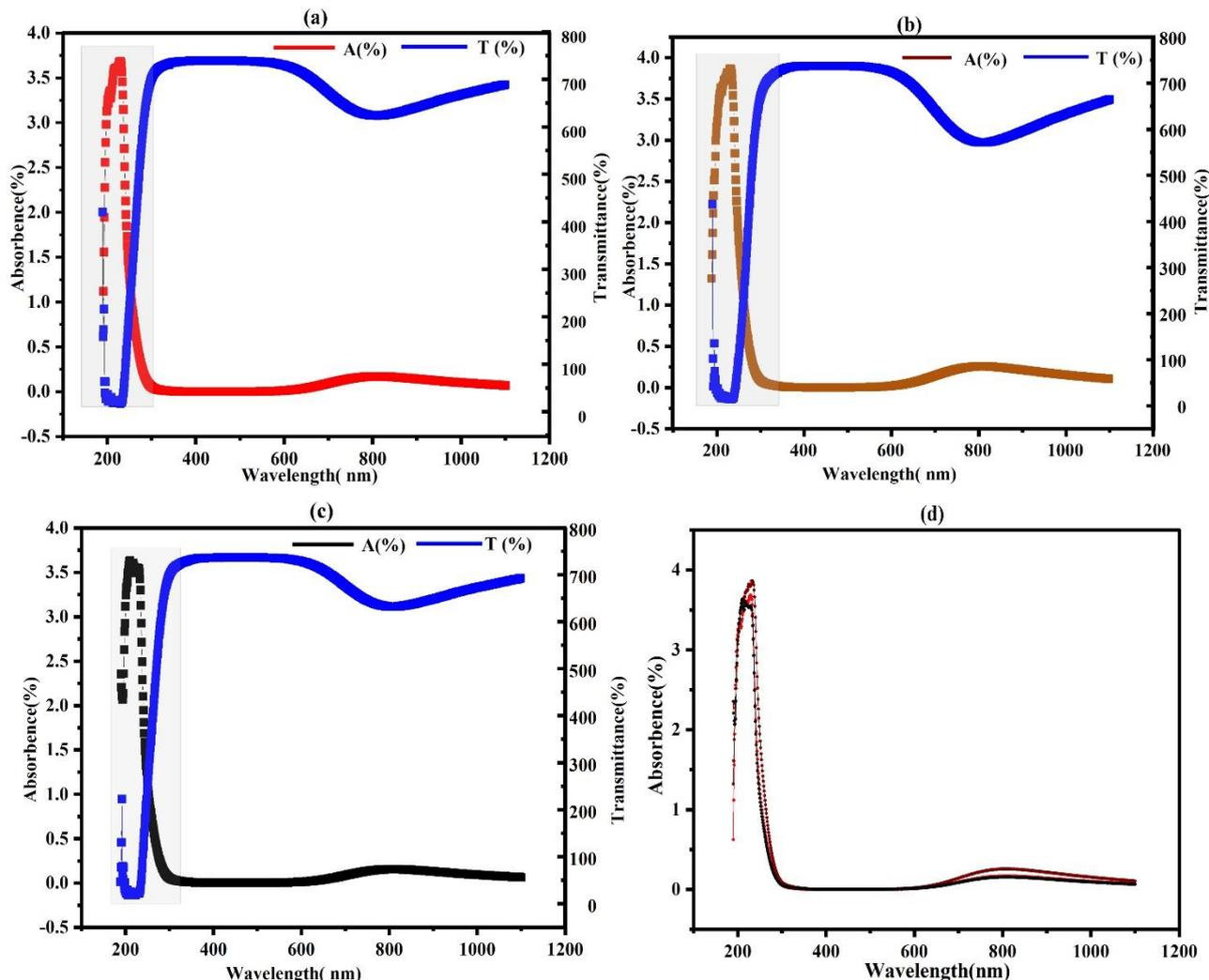
**Figure 6.** Absorption and transmittance spectrum of (a)Laser ,(b) Compact fluorescent lamp, (c) without radiation and (d) The overall changes in absorbance at different conditions.
