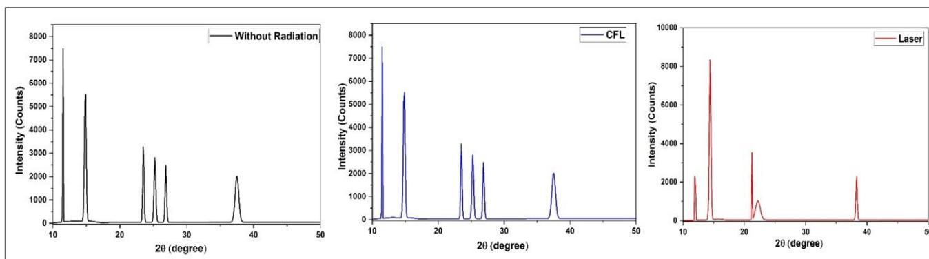
**Figure 3.** X-ray diffractograms of MgCT crystals.
