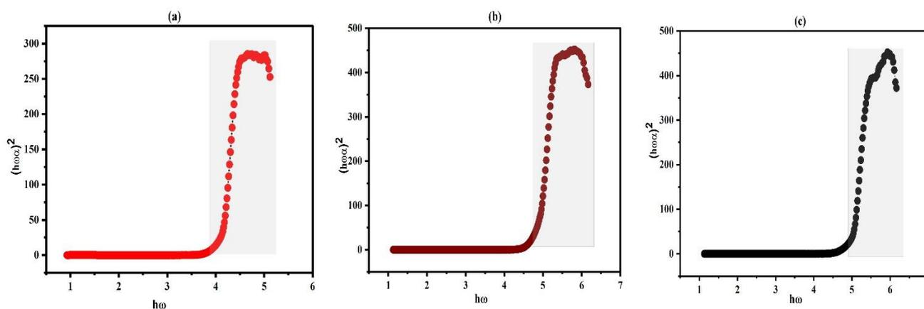
**Figure 7.** Tauc's graph plot between  $(\alpha h\nu)^2$  and the photon energy ( $h\nu$ ) of (a) Laser, (b) Compact fluorescent lamp, (c) without radiation.
