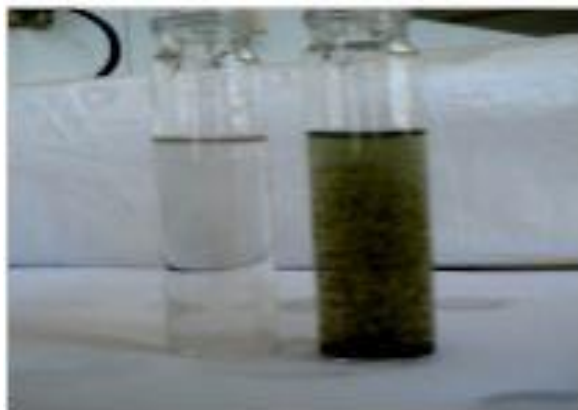
Figure 5. Application of Fenton process of the industrial effluent ( pH=4, [H_2O_2]/[FeSO_4]= 41 , T=40^\circ C )
