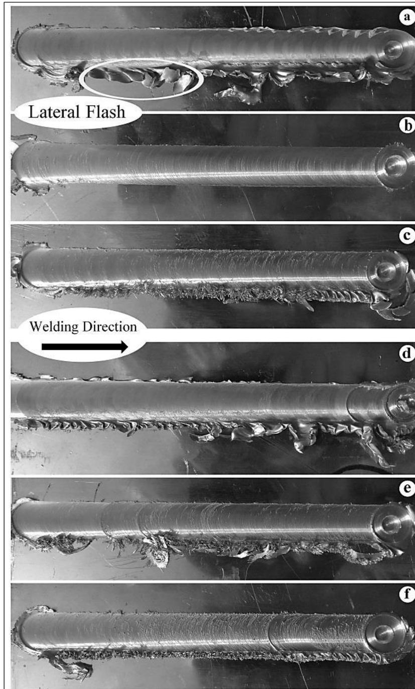
**Figure 2.** The surface of FSW joints.
