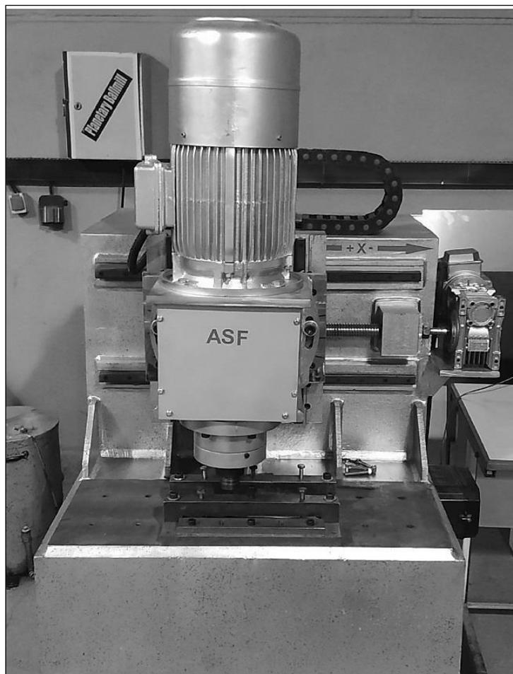
**Figure 1.** The FSW machine applied in the present study
