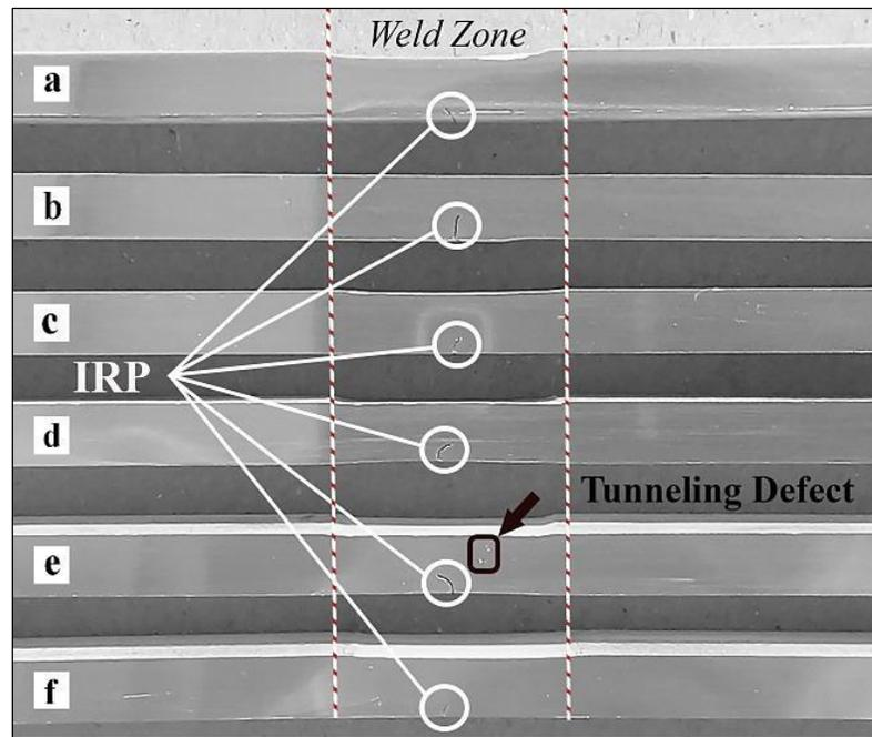
**Figure 3.** The cross-section surface of welding joints
