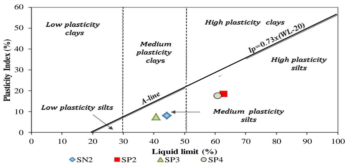
**Figure 5:** Casagrande chart classification of lateritic soils in the study area.
