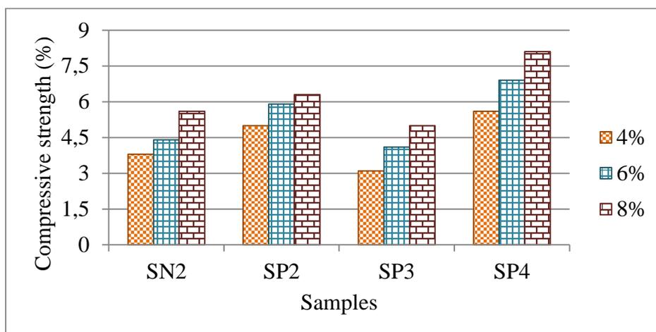
**Figure 6:** Comparative result of compressive strength of common laterite-cement block and in Garoua with earth of varied cement content
