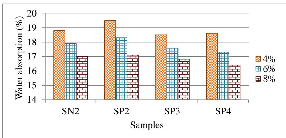
**Figure 7:** Initial rate of water absorption for different percentages of cement
