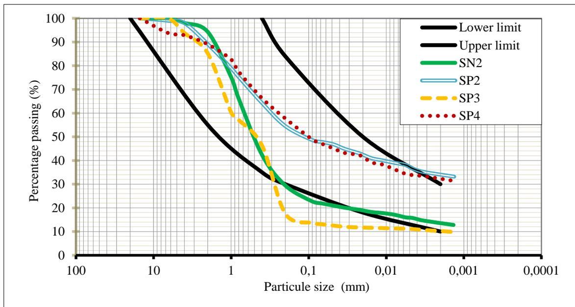
**Figure 4:** Grain size distribution curves, the lower limit and upper limit was established in according with Cameroonian Standards [44].
