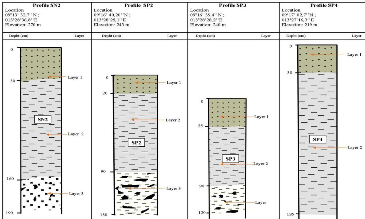
Figure 2: Schematic representations of the studied lateritic soils profile
