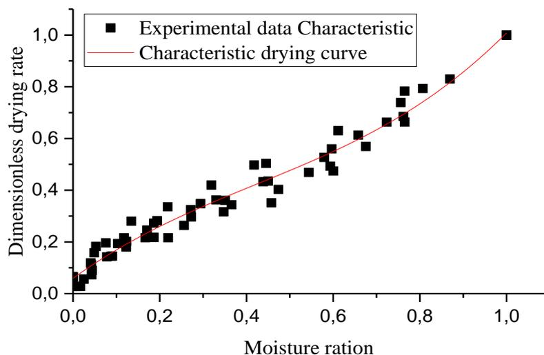
**Figure 4:** Characteristic drying curve of the *Taraxacum Officinale* root
