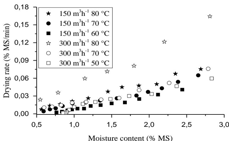
Figure 3: The variation of the drying rate in function of the moisture content
