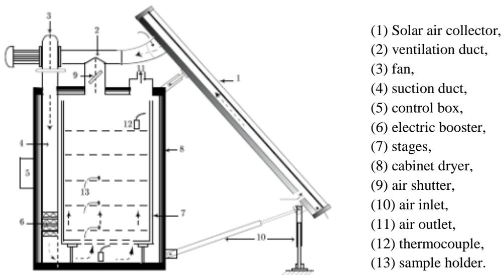
**Figure 1:** The forced convective solar dryer implemented in ENS, Marrakech
