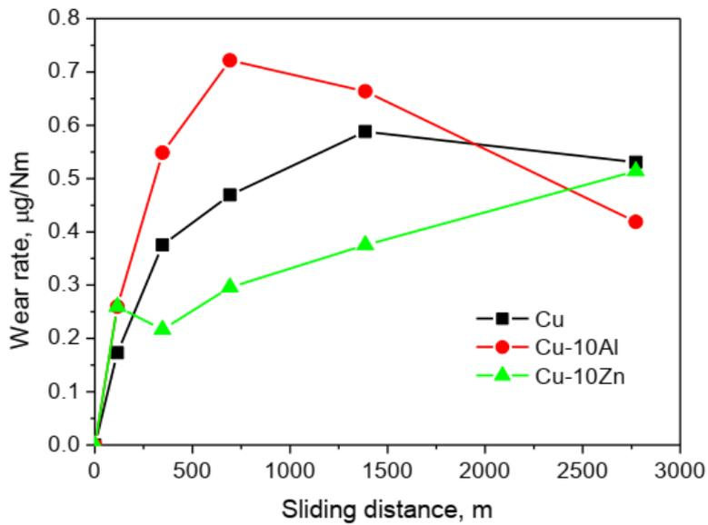
**Figure 4:** Variation of wear rate with the sliding distance in wet sliding condition.
