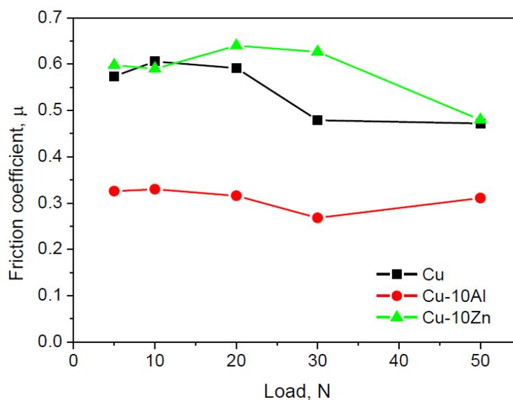
**Figure 9:** Variation of friction coefficient with applied load distance in dry sliding condition
