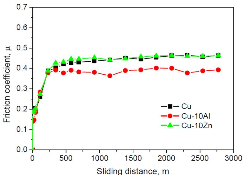
**Figure 7:** Variation of friction coefficient with the sliding distance in wet sliding condition.
