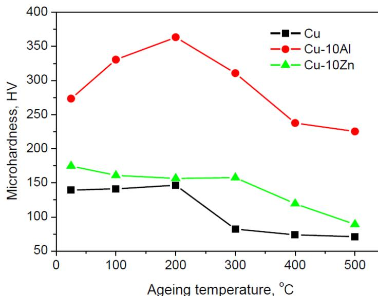
**Figure 1:** Isochronal ageing curve of the 40% cold rolled alloys, aged for 1 hour
