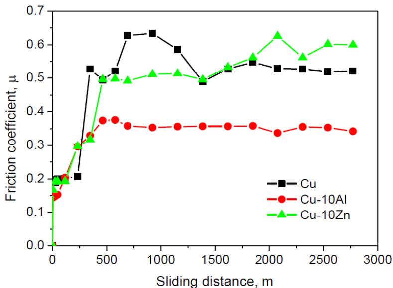
**Figure 6:** Variation of friction coefficient with the sliding distance in dry sliding condition.
