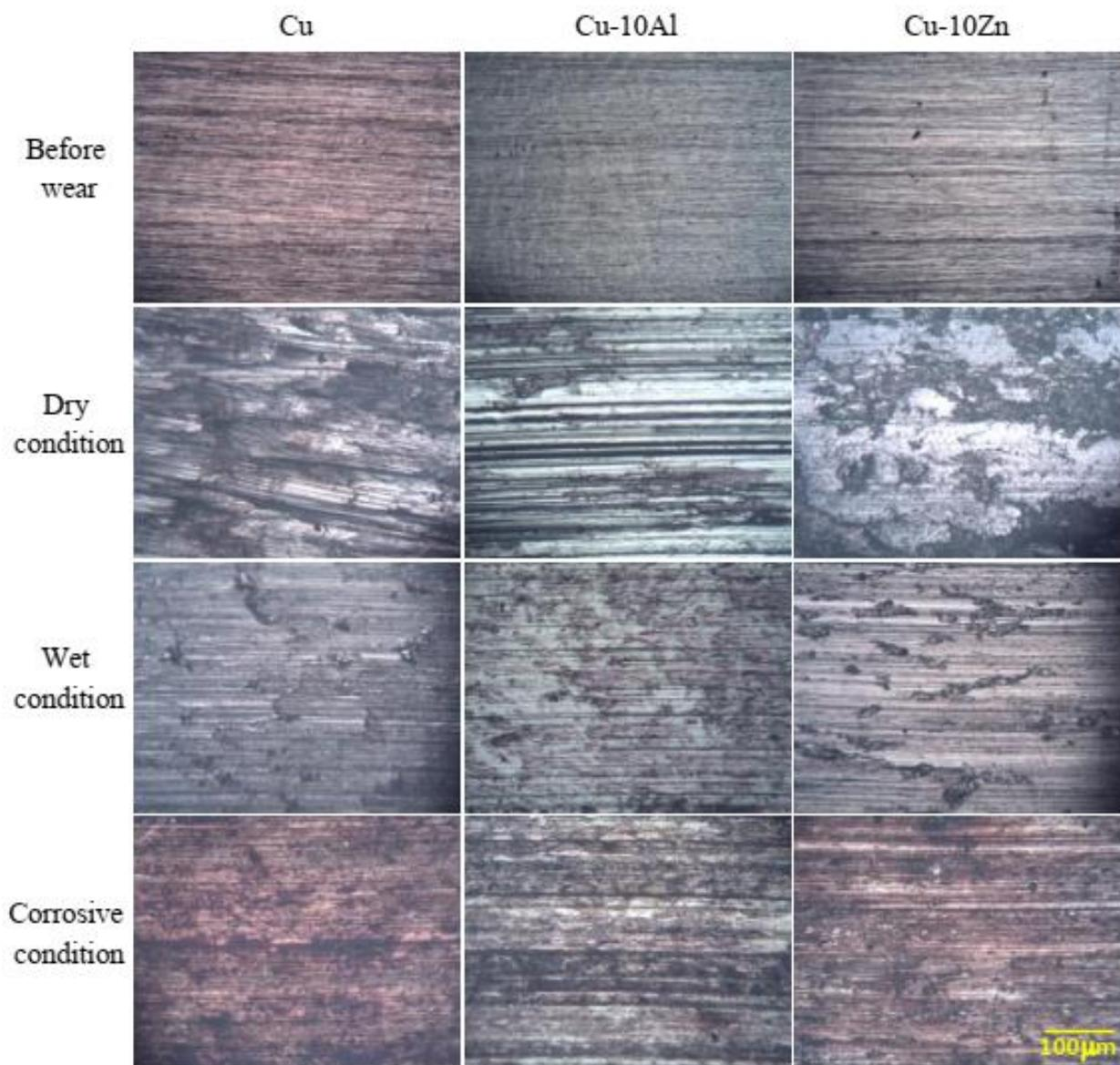
**Figure 12:** Optical micrograph of worn surfaces of Cu, Cu-10Al and Cu-10Zn alloys before wear, after wear for 2772m at applied pressure of 1.02MPa (Load = 20N) and sliding velocity of  $0.385 \text{ ms}^{-1}$  in dry, wet and corrosive sliding condition
