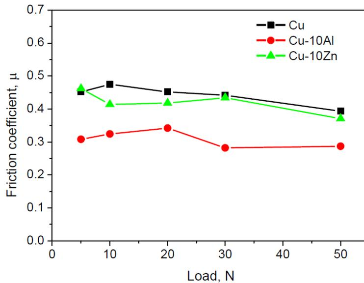
**Figure 10:** Variation of friction coefficient with applied load distance in wet sliding condition
