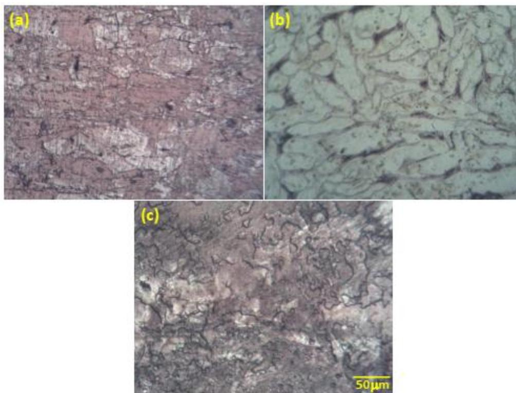
**Figure 13:** Optical micrograph of 40% cold-rolled alloys (a) Cu (b) Cu-10Al and (c) Cu-10Zn alloys aged at 200°C for one hour
