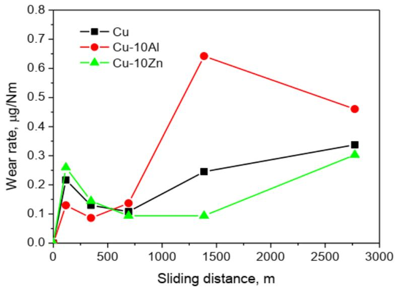
**Figure 3:** Variation of wear rate with the sliding distance in dry sliding condition.
