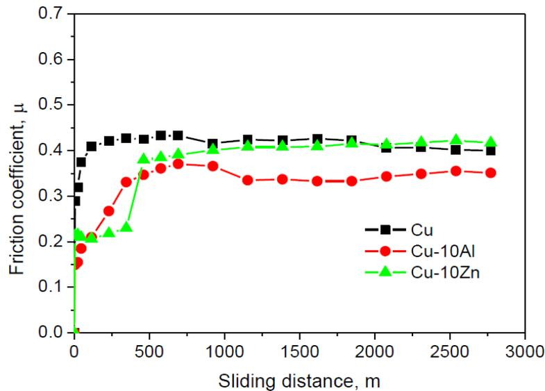
**Figure 8:** Variation of friction coefficient with the sliding distance in corrosive sliding condition.
