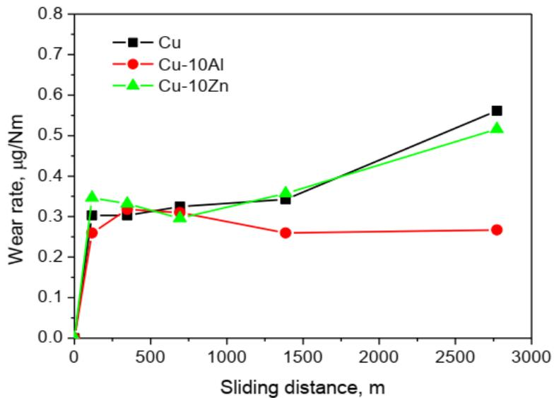
**Figure 5:** Variation of wear rate with the sliding distance in corrosive sliding condition.
