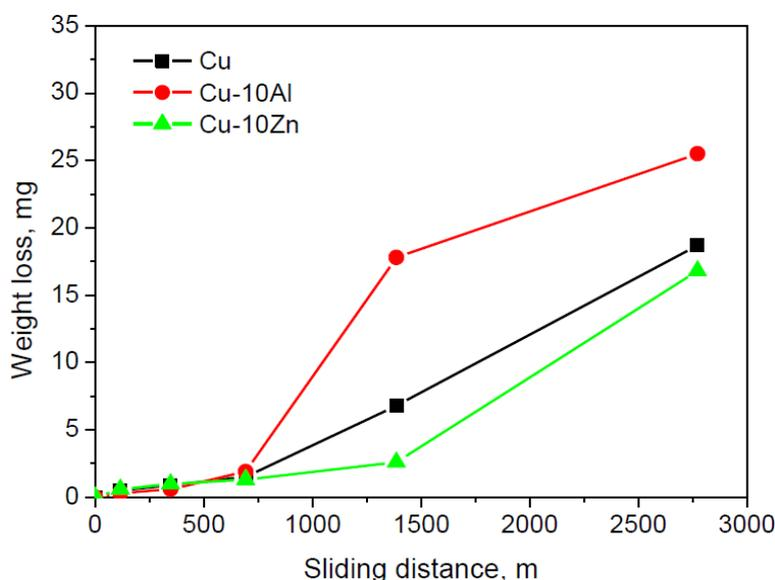
**Figure 2:** Variation of weight loss with the sliding distance in dry sliding condition
