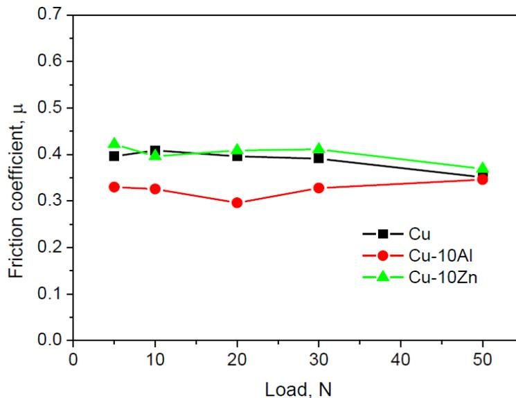
**Figure 11:** Variation of friction coefficient with applied load distance in corrosive sliding condition
