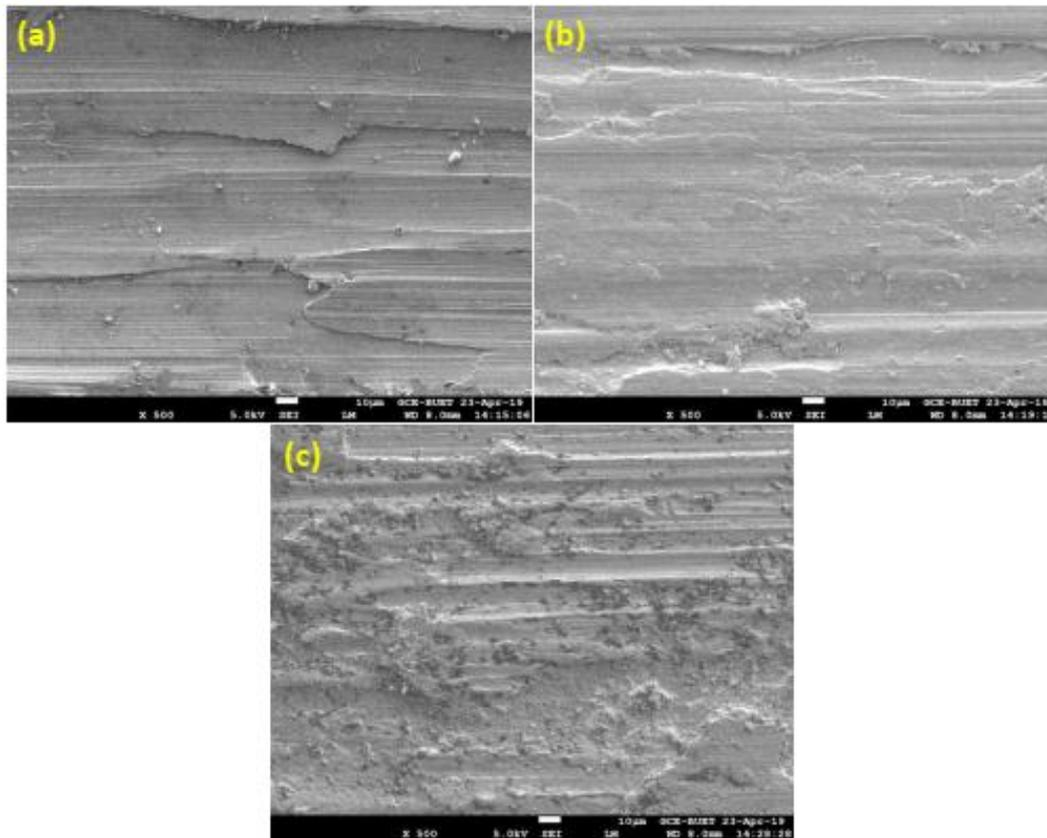
**Figure 14:** SEM images of the worn surfaces of the a) Cu, b) Cu-10Al and c) Cu-10Zn alloy after wear for 2772m at applied pressure of 1.02MPa (Load = 20N) and sliding velocity of 0.385 ms<sup>-1</sup> in dry sliding condition
