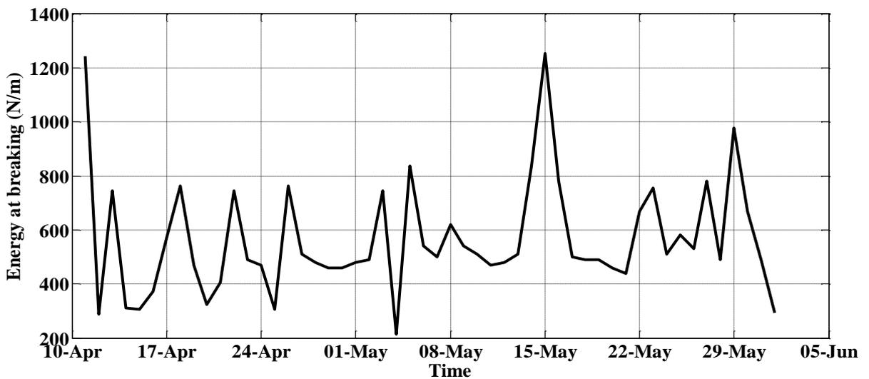
**Figure 5:** Significant wave energy at breaking estimated in April and May 2018
