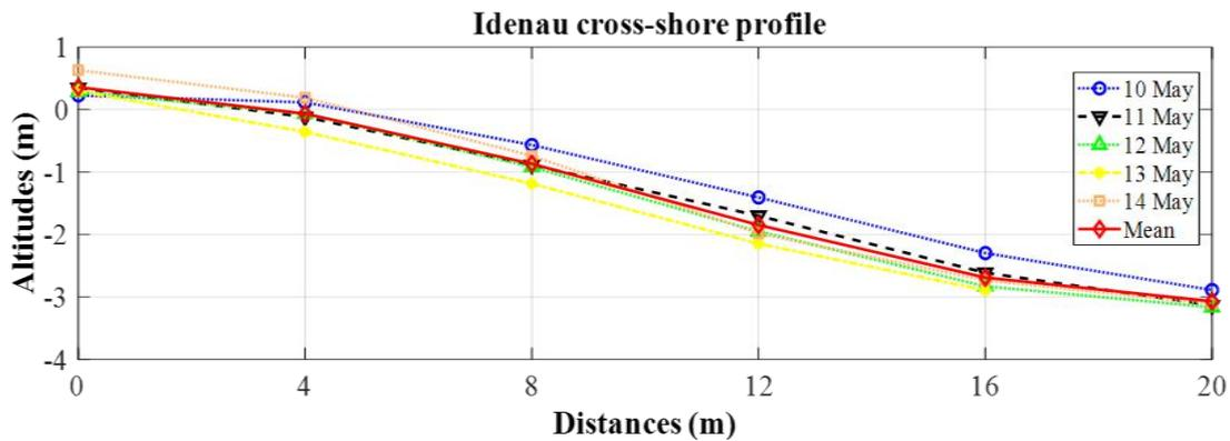
**Figure 9:** Evolution of topographic profiles of Idenau beach
