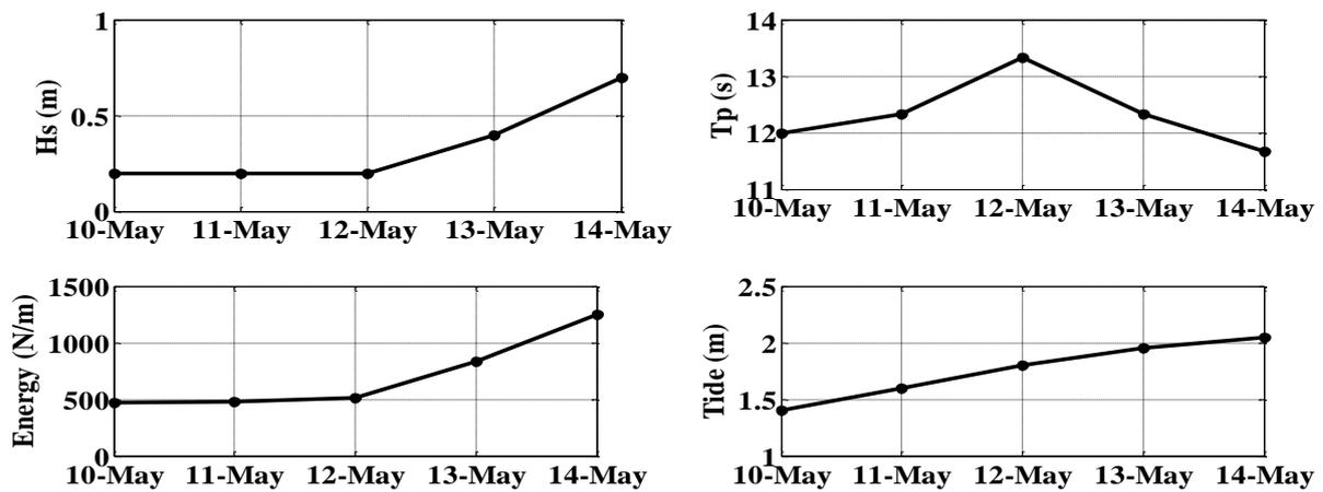
**Figure 11:** Hydrodynamic forcings during the study period (10<sup>th</sup> May to 14<sup>th</sup> May): Significant wave height (top of the left), Peak period (top of the right), Energy (bottom of the left) and Tidal (bottom of the right).
