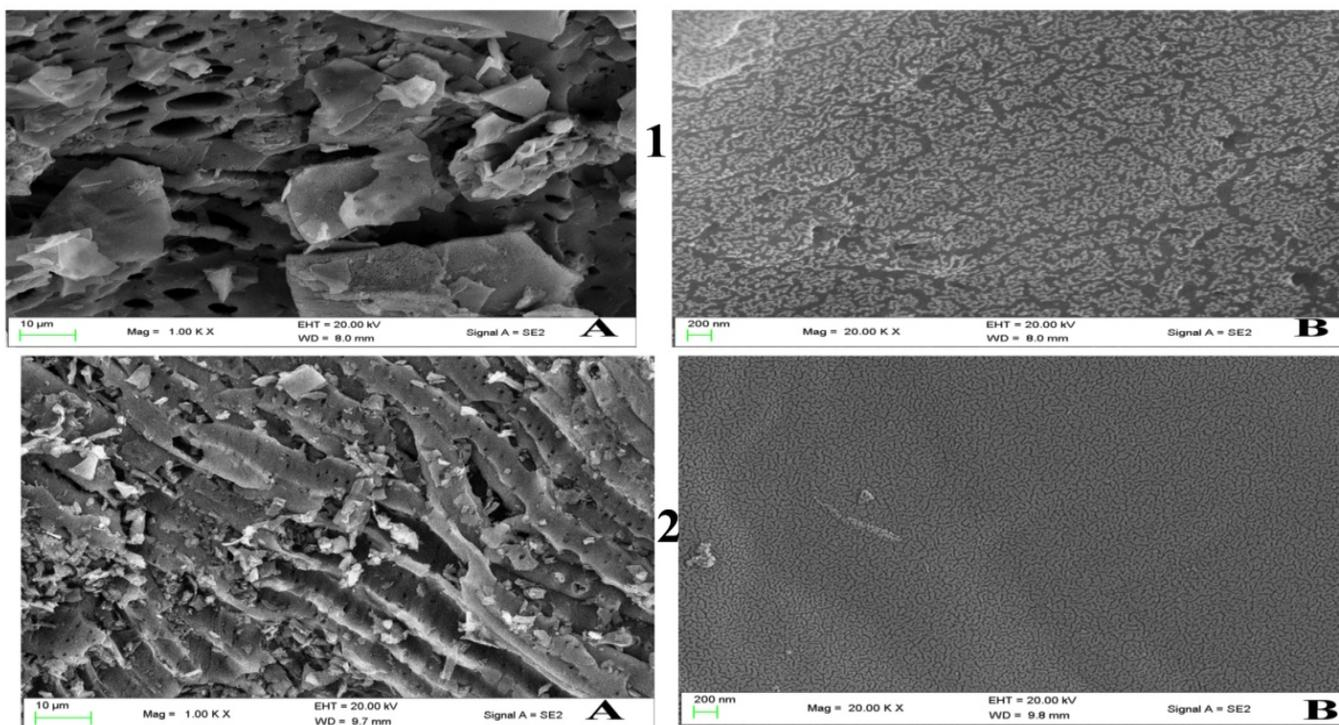
**Figure 2:** Scanning electron micrographs of groundnut shell activated with Zinc Chloride GZAC (1) and  $\text{H}_3\text{PO}_4$ GPAC (2) at 10  $\mu\text{m}$  (A) and 200 nm (B).
