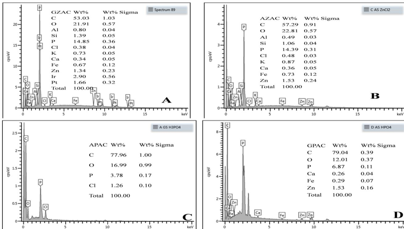
**Figure 4:** EDX spectra of AC produced by activating with Zinc Chloride; for groundnut (GZAC) (A), for Almond AZAC (B) and AC produced by activating with Phosphoric acid; for Almond (APAC) (C), for groundnut GPAC (D)
