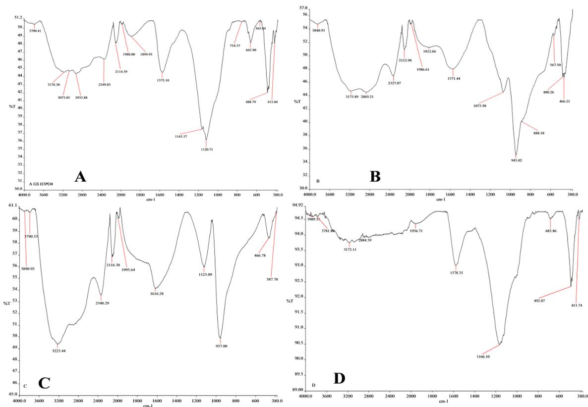
**Figure 1:** FTIR result of the produced activated carbon from Groundnut and almond shell using Phosphoric acid (A & C) and Zinc Chloride (B & D) as activating agent.
