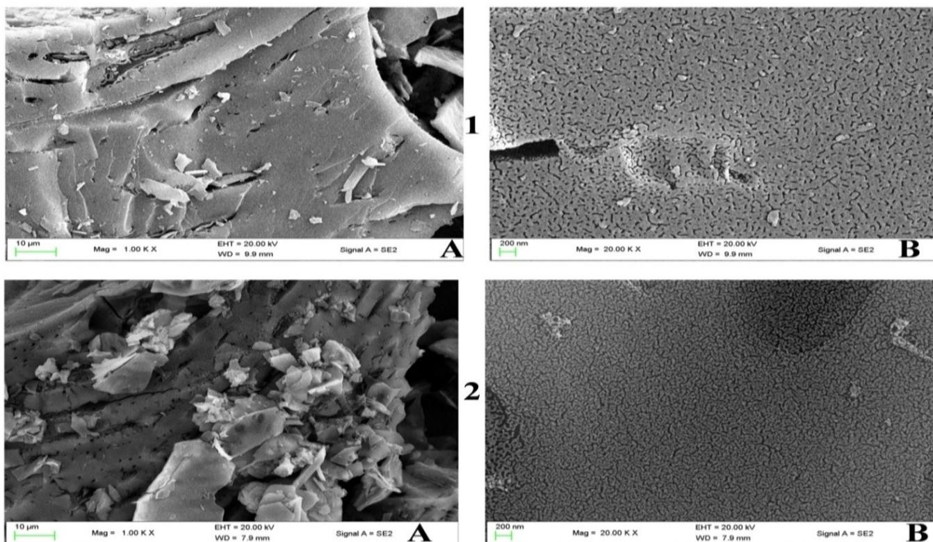
**Figure 3:** Scanning electron micrographs of almond shell activated with  $\text{H}_3\text{PO}_4$  APAC (1) and Zinc Chloride AZAC (2) at 10  $\mu\text{m}$  (A) and 200 nm (B).
