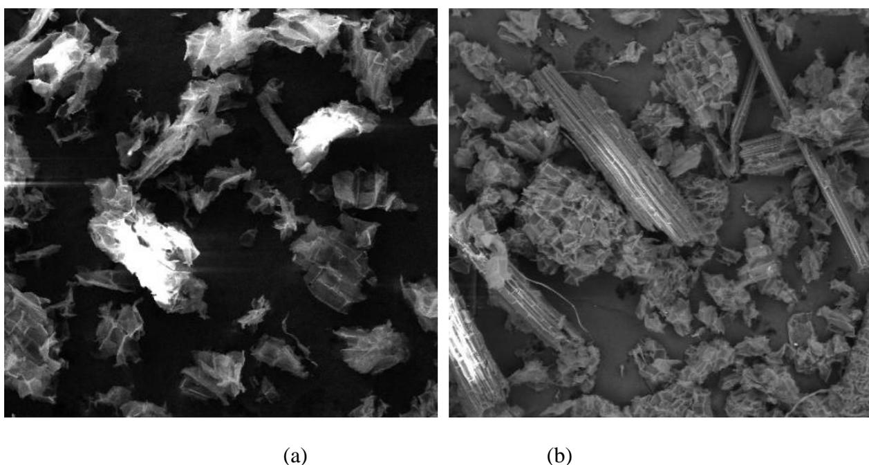
**Figure 4:** Morphology of the SB-KOH by SEM analysis with magnification (a-70x,b-50x)
