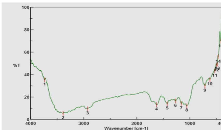
Figure 3: FTIR spectrum of Treated *Sugarcane Bagasse* (SB-KOH) before adsorption.
