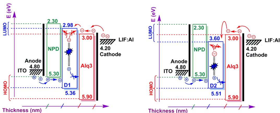
Fig. 12: Typical OLEDs architecture including **D1** and **D2** as emitting layers.
