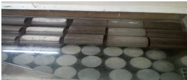
**Figure 5:** Conservation of concrete specimens.
