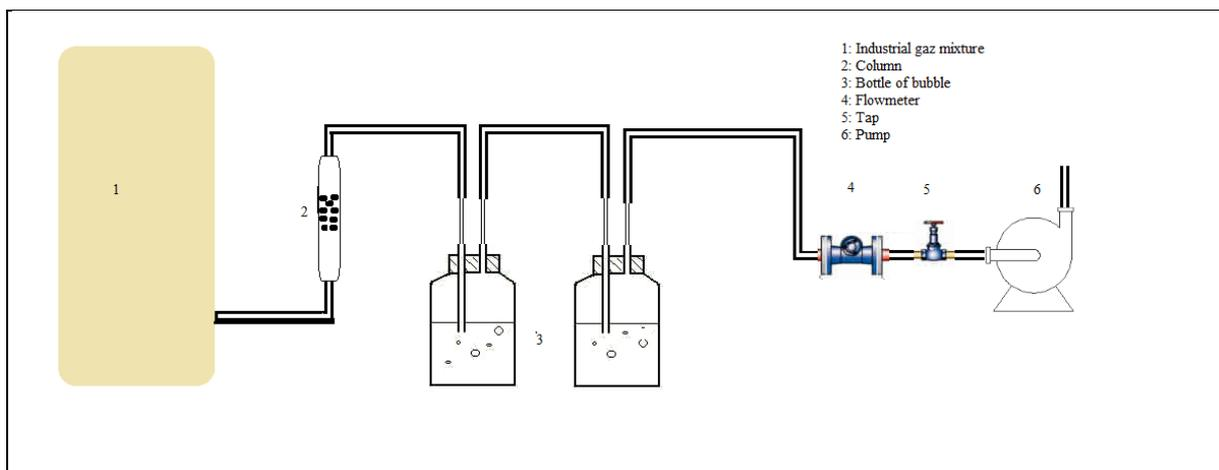
**Figure 1:** Experimental set-up for H<sub>2</sub>S adsorption tests
