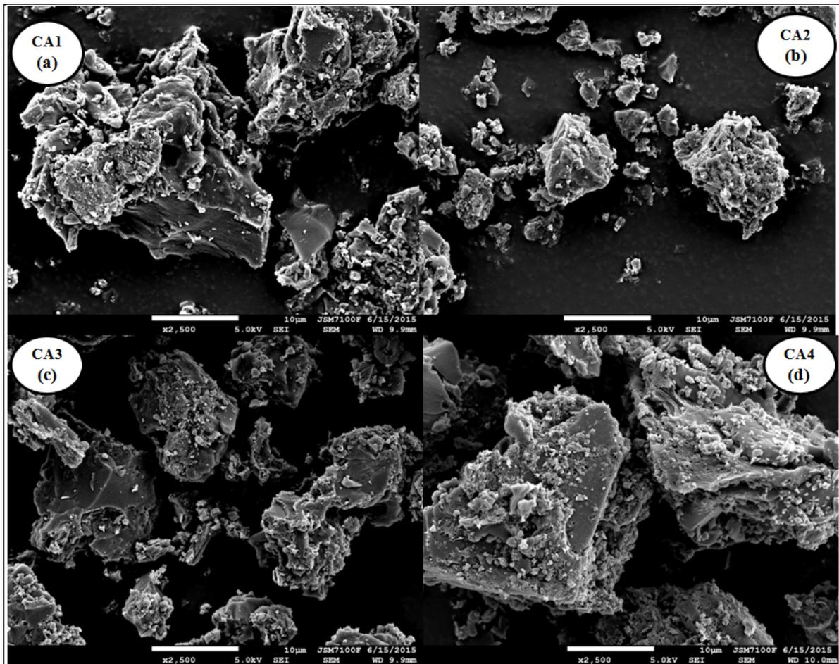
**Figure 3:** SEM images of the 4 activated carbon.
