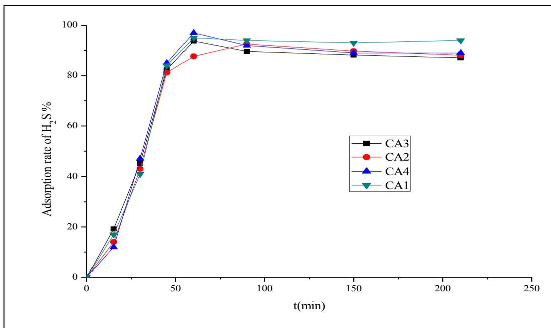
**Figure 4:** Adsorption capacity of H<sub>2</sub>S by activated carbon
