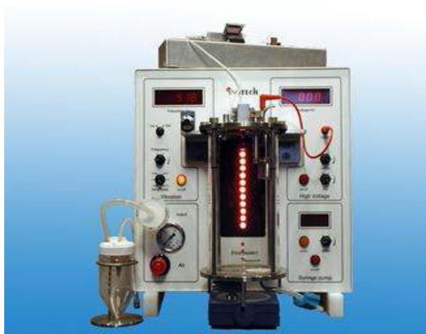
**Figure 1** Encapsulator for making uniform gel beads
