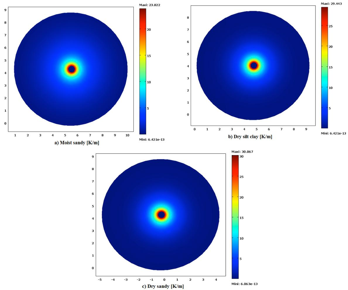
**Figure 8:** Surfaces of temperature gradients in each soil
