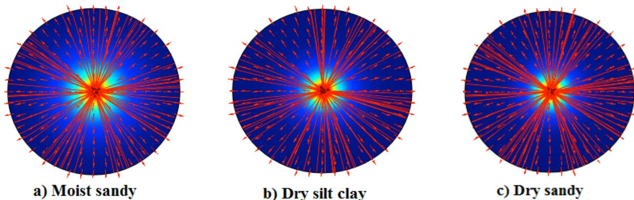
Figure 12: Superposition of temperature and heat flow
