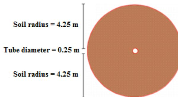
Figure 1: Geometry of soils studied on comsol
