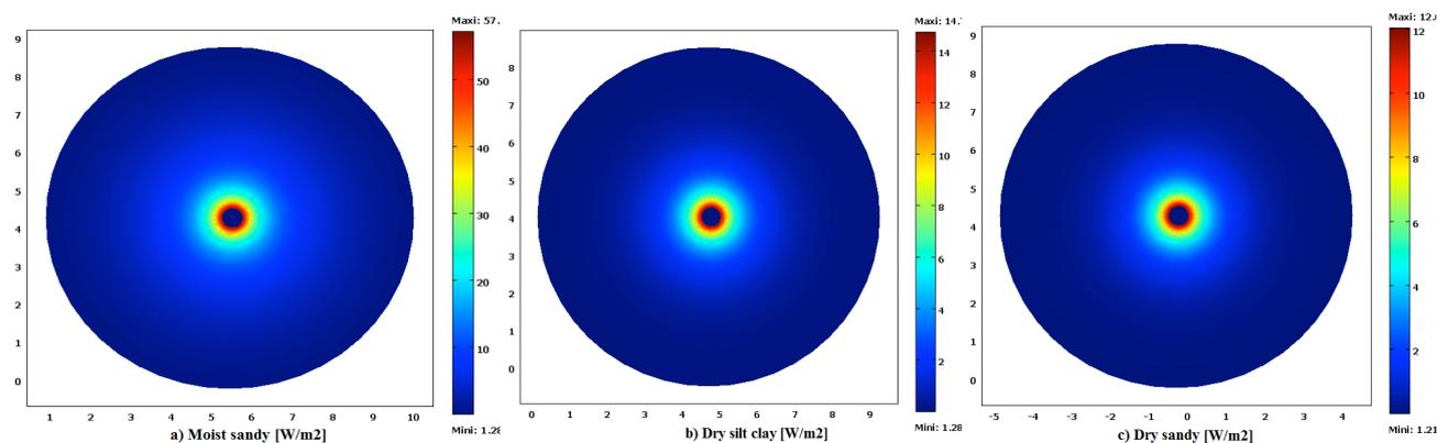
Figure 11: Surfaces of heat flow diffused in each soil
