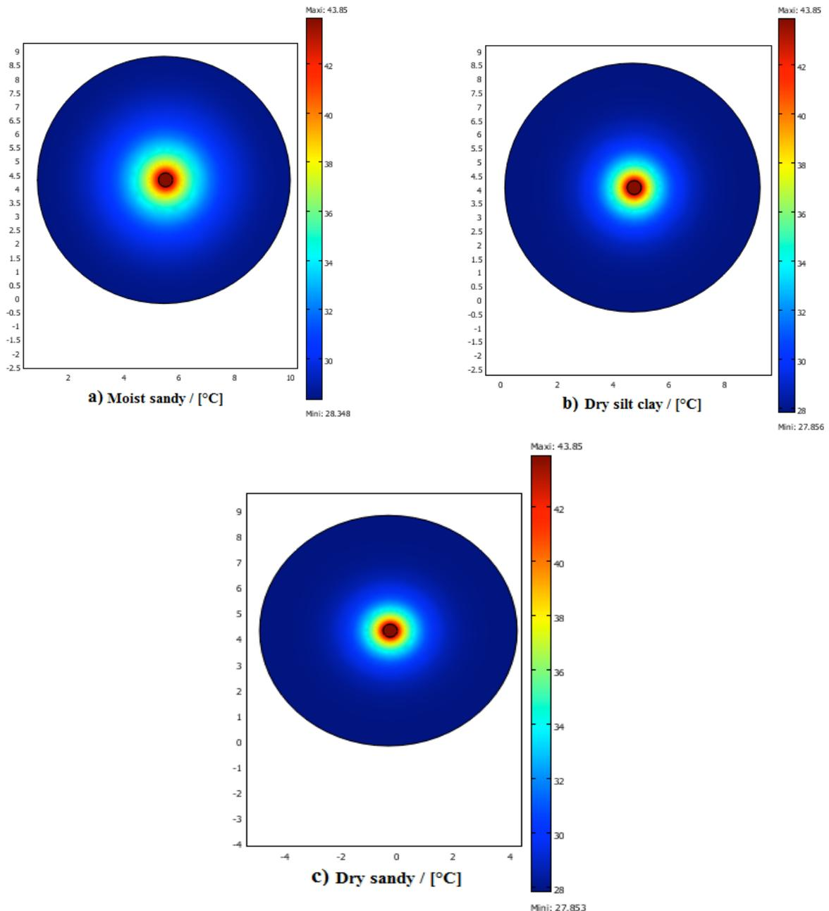
**Figure 6:** Temperature surfaces in each soil
