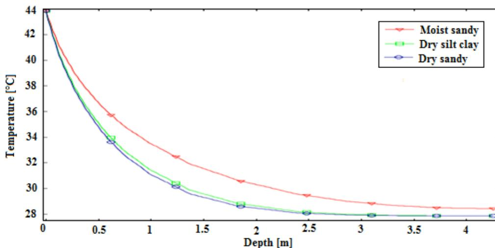
**Figure 13:** Evolution of the temperature of three different soils
