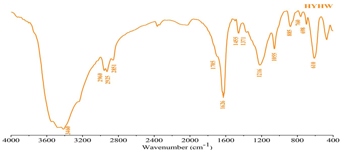
**Figure 6:** FT-IR spectrum of oil shale extract.
