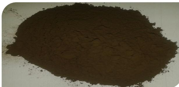
Figure 2: Fully-crushed oil shale.
