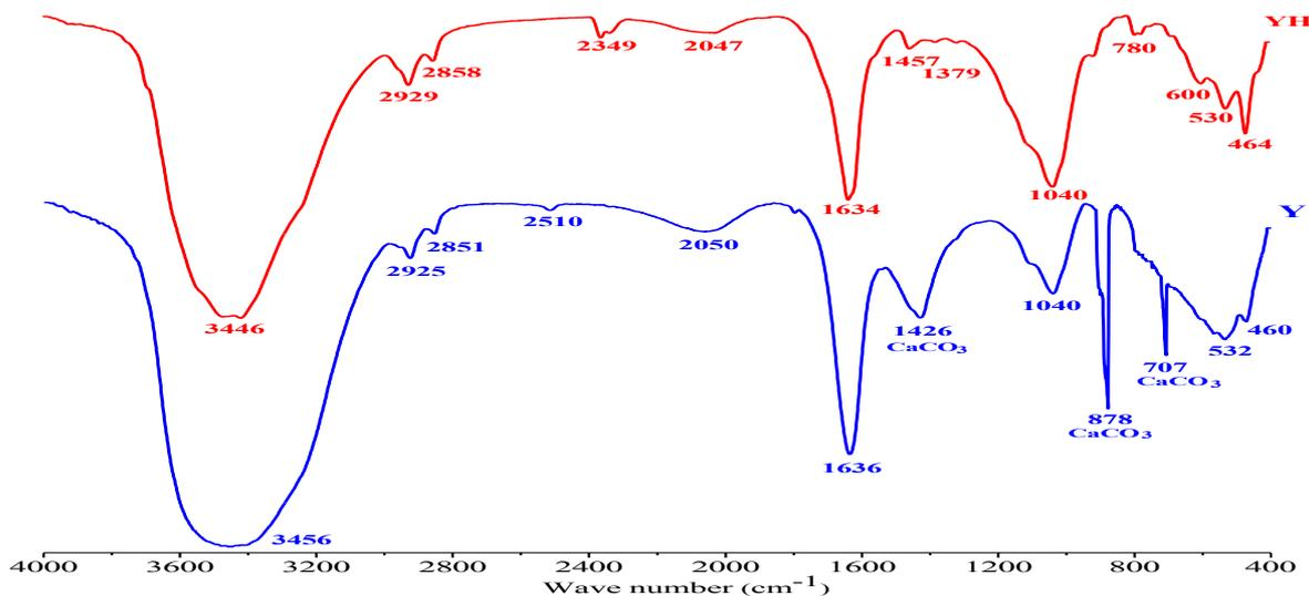
**Figure 4:** FT-IR spectrum of raw oil shale (Y) and the oil shale decarbonized (YH).
