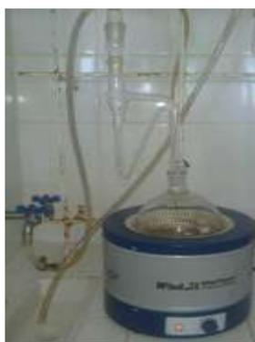
**Figure 2:** Assembly of extraction of essential oils by the hydro-distillation method.
