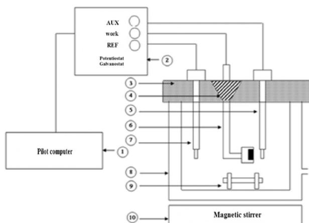
**Figure 1:** Experimental setup. 1 - Pilot computer 2 - Potensiostat-galvanostat 3 - Cover electrode holder 4 - Cap sample holder 5 - Platinum electrode 6 - Sample: steel pelle XC10 (1.003 cm) embedded in an inert resin 7 - Reference electrode Calomel saturated KCl 8 - Glass beaker of 600 mL 9 - Magnetic bar 10 - Magnetic stirrer.
