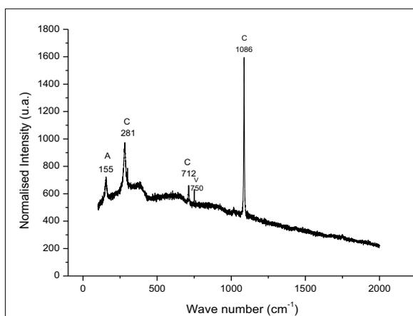
**Figure 18:** Raman spectra of precipitated scale products in presence of 0.5mg/L of K<sub>2</sub>HPO<sub>4</sub>.
