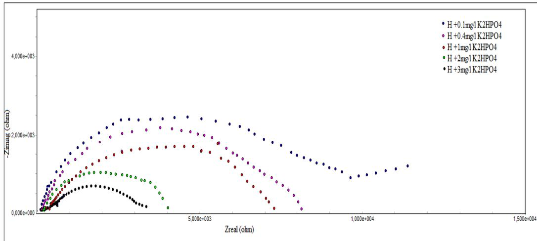
**Figure 5:** Impedance diagrams obtained for treated water of Hamma at different concentrations of  $K_2HPO_4$ (T=30°C).
