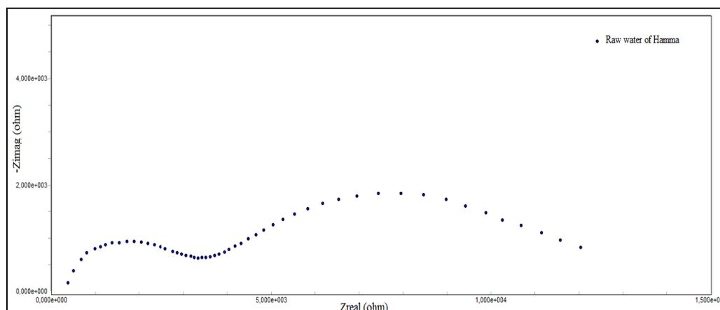
**Figure 4:** Impedance diagram obtained for raw water from Hamma.
