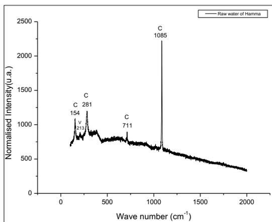
**Figure 16:** Raman spectra of Hamma raw water.
