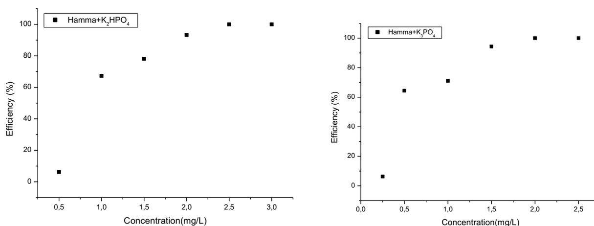
**Figure 12:** Evolution of the efficiency as a function of the concentration of K<sub>2</sub>HPO<sub>4</sub> and K<sub>3</sub>PO<sub>4</sub> in Hamma water
