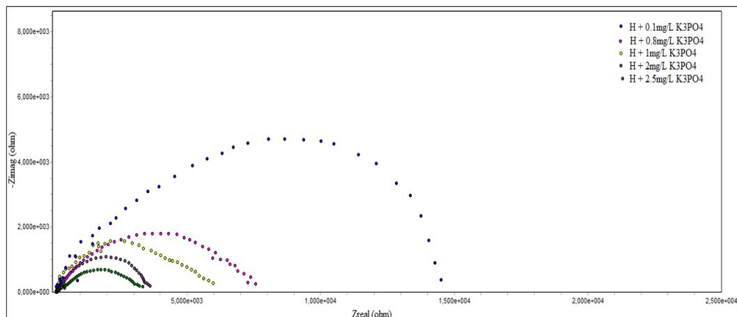
**Figure 6:** Impedance diagrams obtained for treated water of Hamma at different concentrations of  $K_3PO_4$ (T=30°C).
