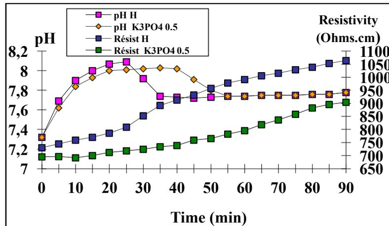
Figure 9: FCP curves of treated Hamma water with 0.5 mg/L of  $K_3PO_4$ .
