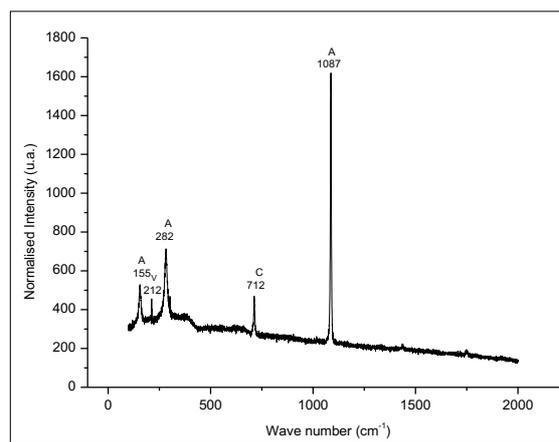
**Figure 17:** Raman spectra of precipitated scale products in presence of 0.5mg/L of K<sub>3</sub>PO<sub>4</sub>.
