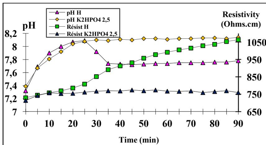
Figure 10: FCP curves of treated Hamma water with 2,5 mg/L of  $K_2HPO_4$ .
