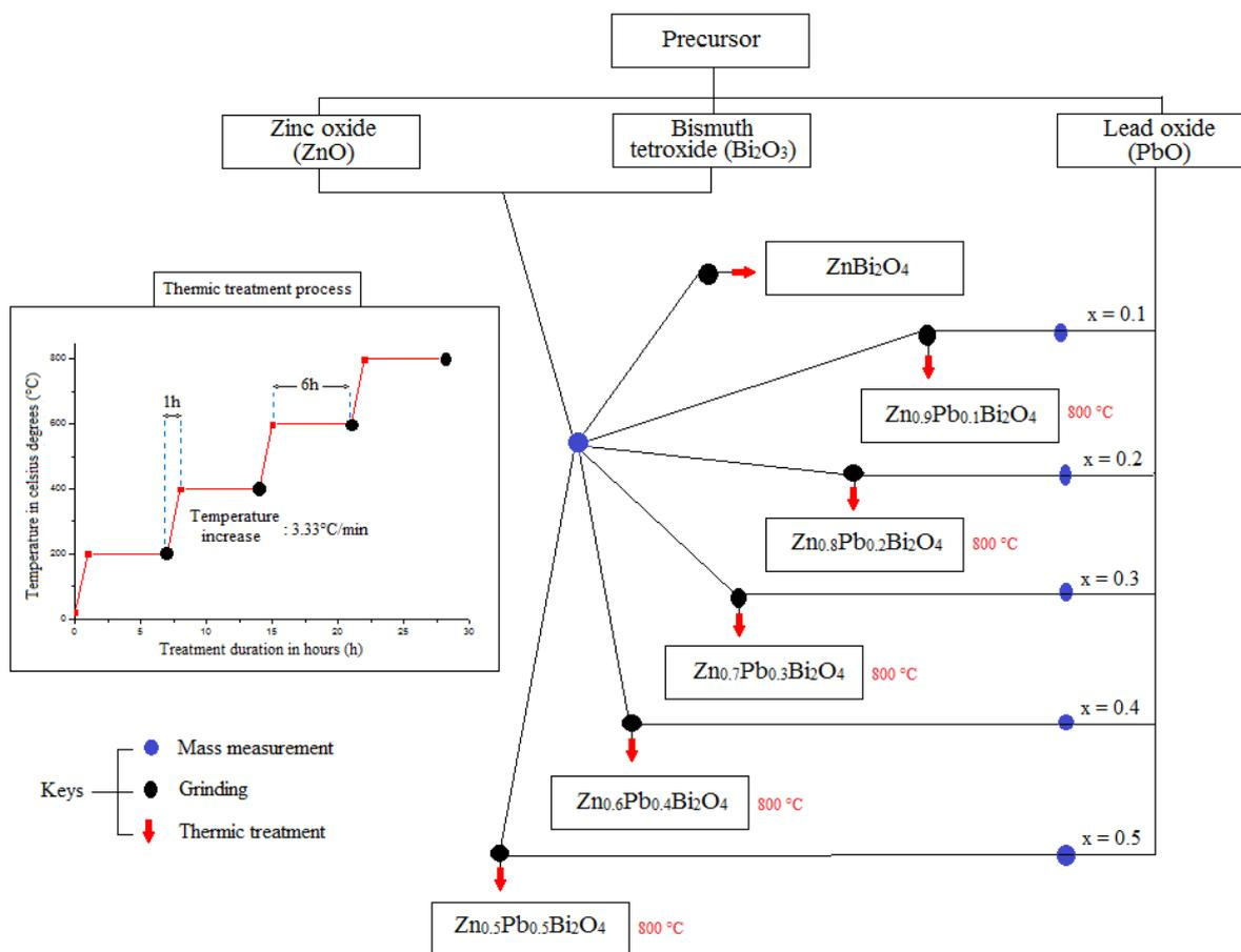
**Figure 1** : Synthesis process for the elaboration of various  $Zn_{1-x}Pb_xBi_2O_4$  ( $x=0.0, 0.1, 0.2, 0.3, 0.4$  and  $0.5$ ) spinels by solid state method.
