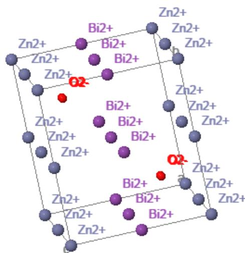
**Figure 2** : Representation of the  $ZnBi_2O_4$  compound.
