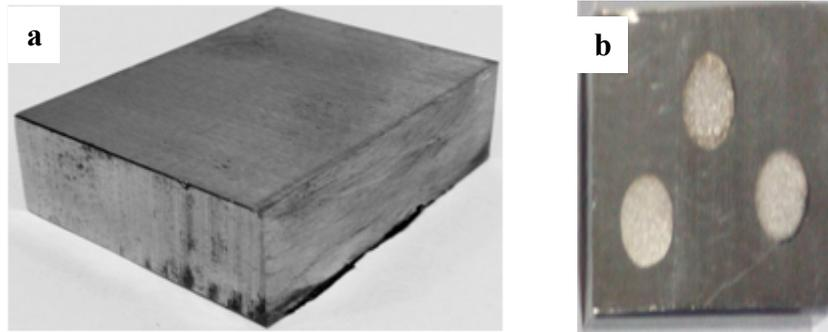
**Figure 3:** AISI D3 die-steel workpiece before and after machining
