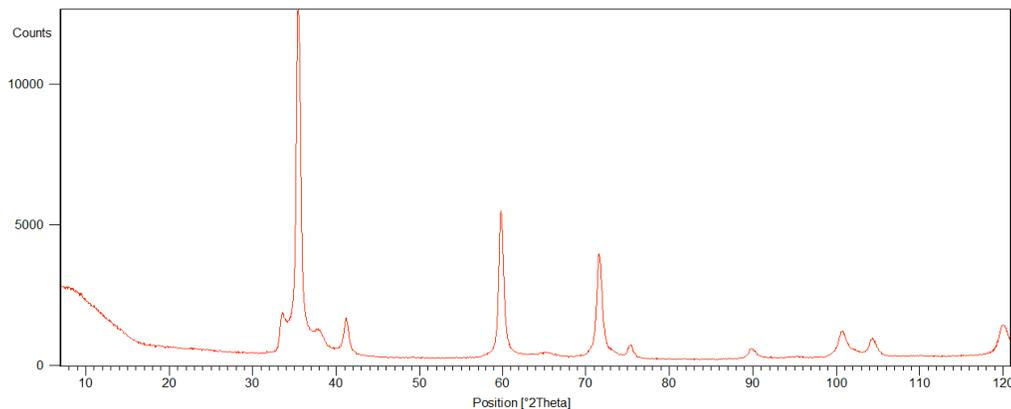
**Figure 5:** SiC nanopowder XRD spectra
