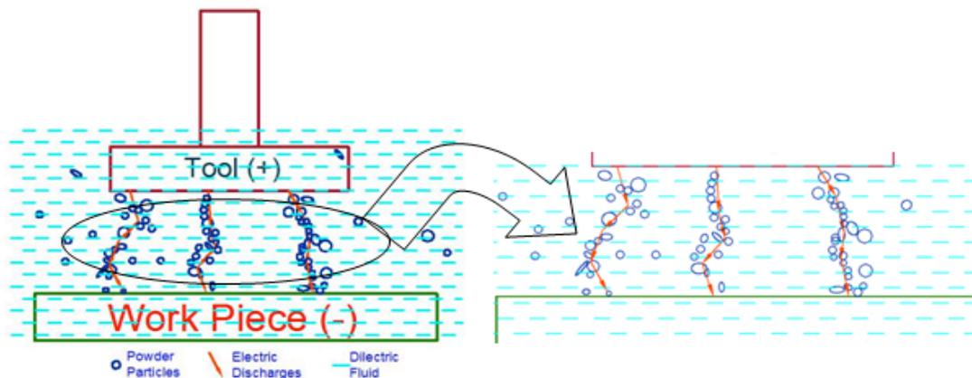
**Figure. 1** Schematic depicting nano powder blended based dielectric EDM technique
