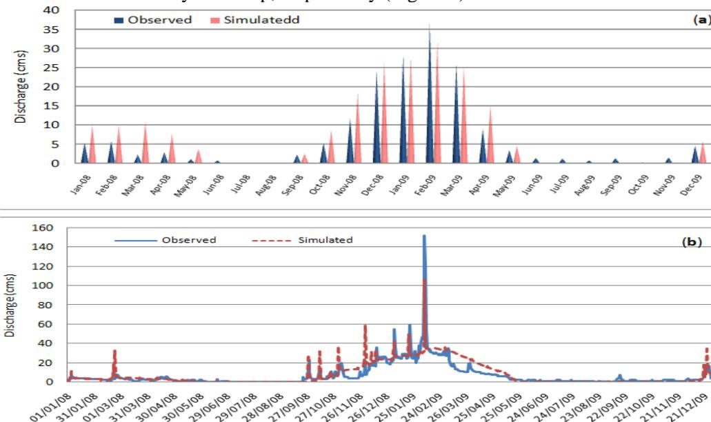
**Figure 6:** Observed Vs predicted monthly (a) and daily (b) discharge during the validation period at the Souk lhad flow gauge
