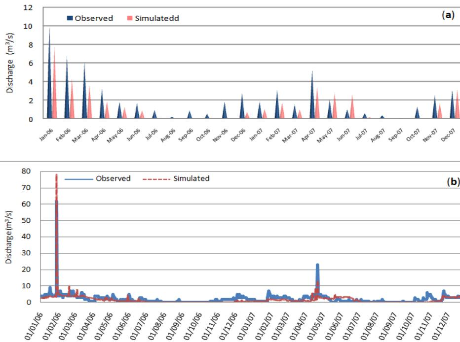
**Figure 5:** Observed vs simulated monthly (a) and daily (b) discharge after manual calibration at the Souk Elhad flow gauge
