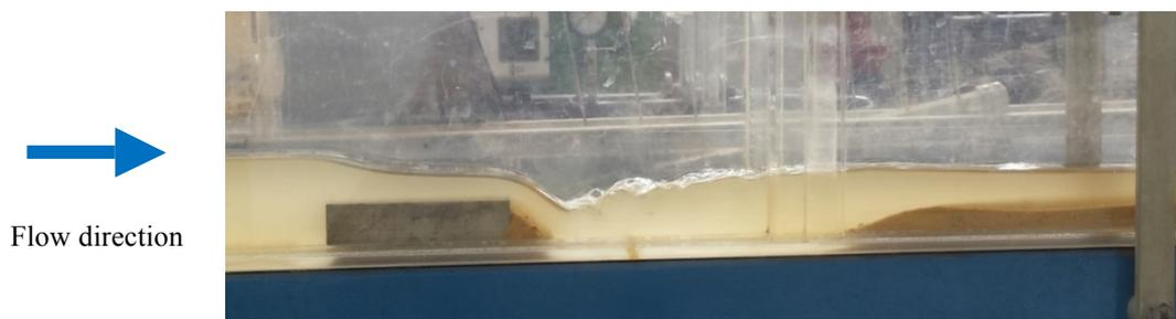
**Figure 5:** Evolution of the sand layer in the channel
