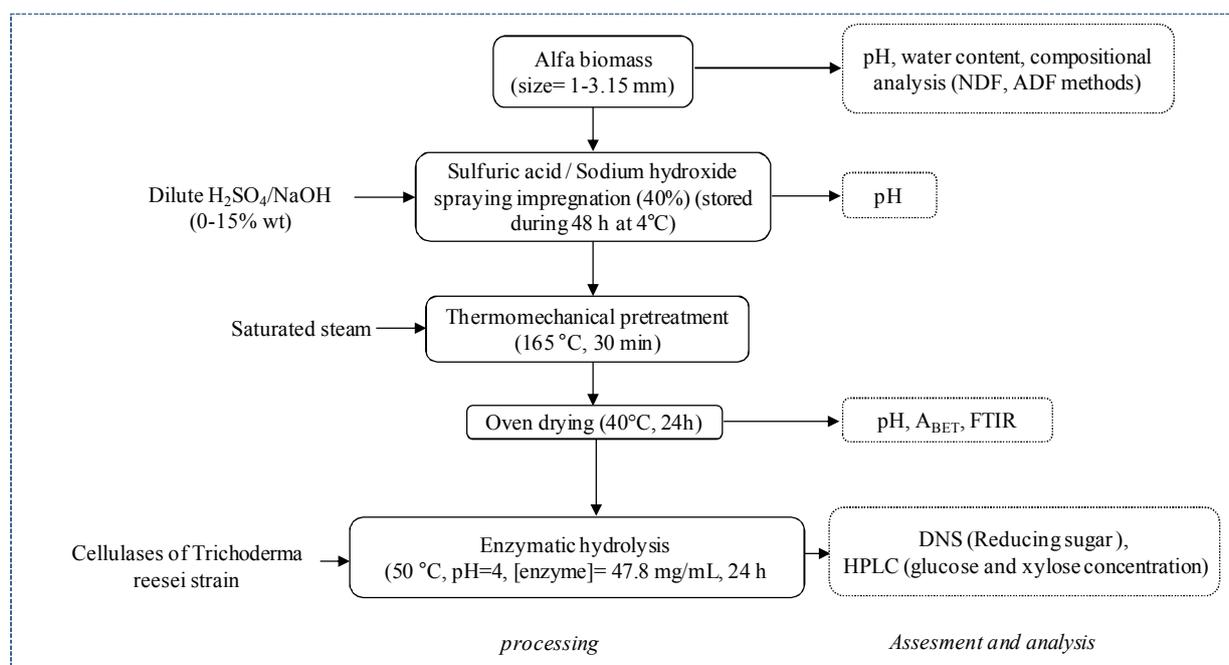
**Figure 2.** Flow chart for the acid or alkali catalyzed combined to DIC process pretreatment.
