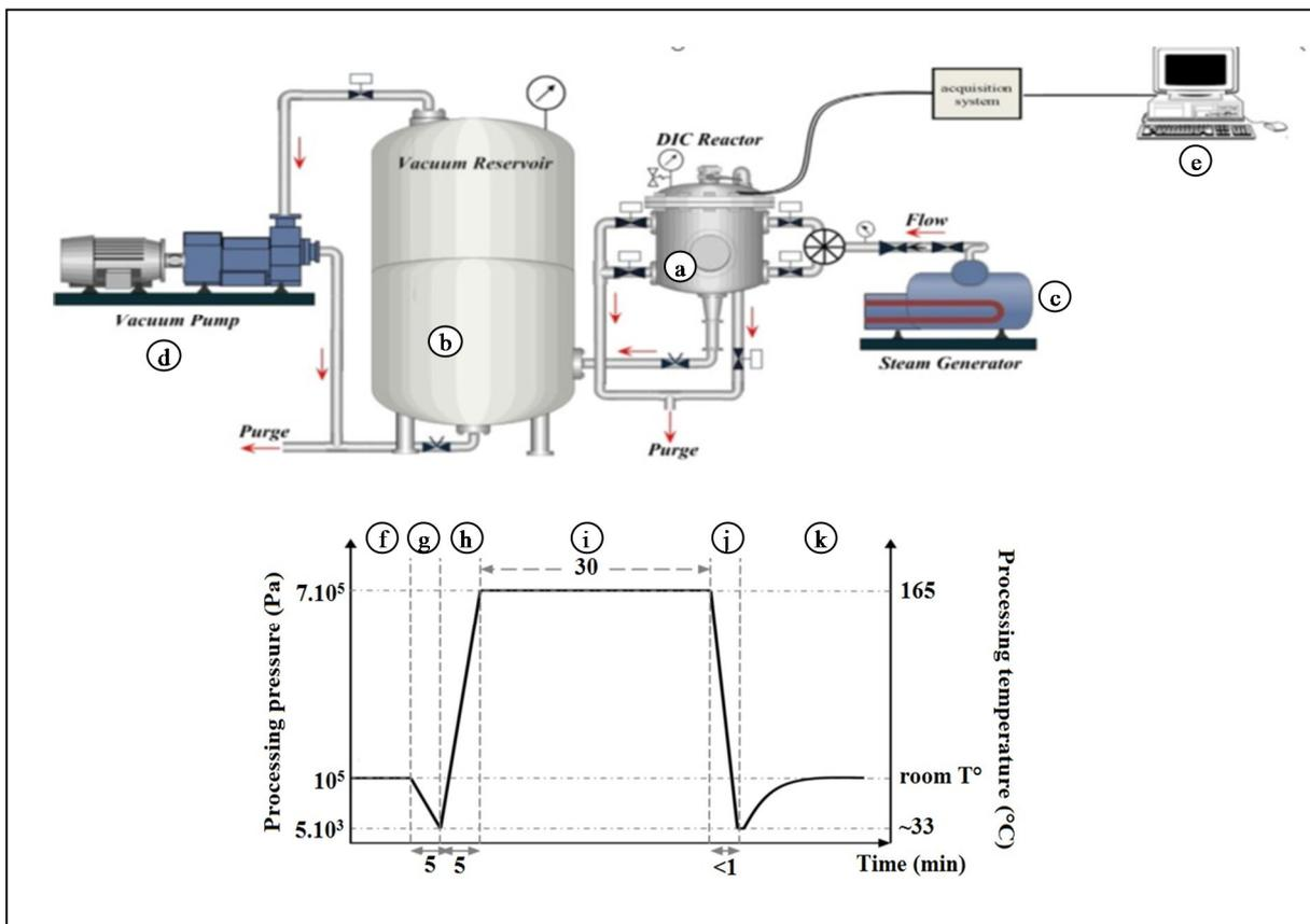
**Figure 1.** Experimental set-up of DIC process and typical pressure-temperature-time profile.
