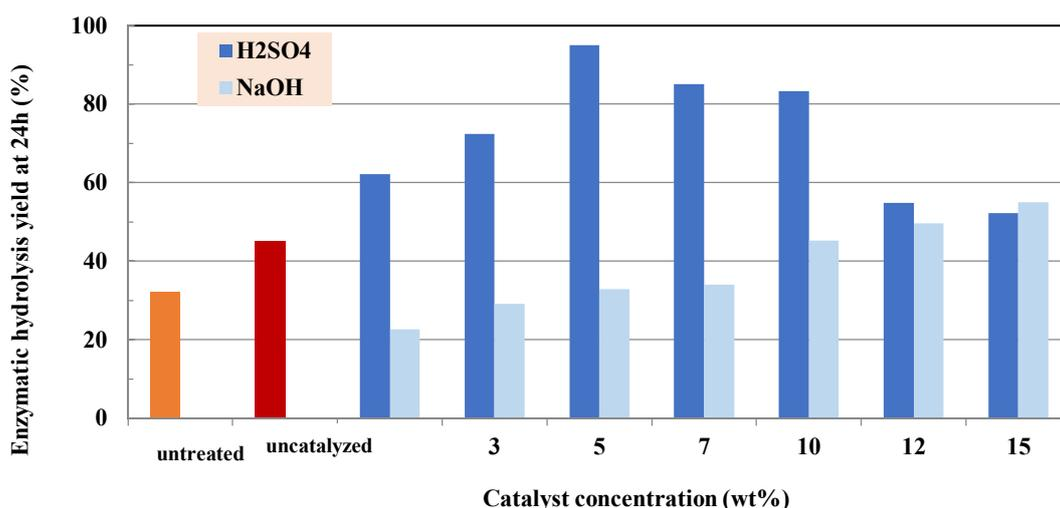
**Figure 5.** Enzymatic hydrolysis yield as function of catalyst concentrations.
