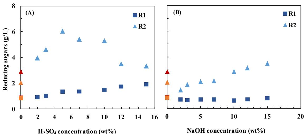
**Figure 4.** Effect of catalyst concentration on reducing sugar release at 0 h (R<sub>1</sub>) and 24 h (R<sub>2</sub>) of enzymatic hydrolysis. (A): H<sub>2</sub>SO<sub>2</sub> and (B): NaOH. The red and orange colors correspond to the uncatalyzed and untreated Alfa, respectively.
