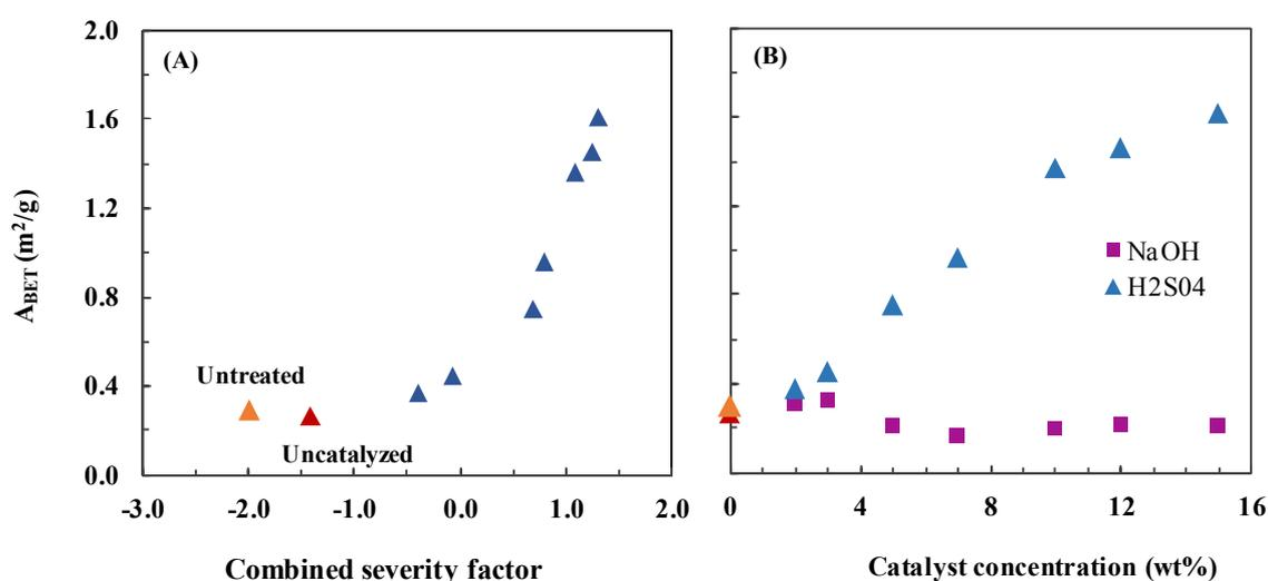
**Figure 3.** Effect of the severity conditions (A) and catalyst concentration (B) on specific surface area of treated Alfa.
