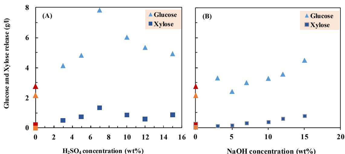
**Figure 6.** Glucose and xylose release after 24 h of enzymatic hydrolysis as function of sulfuric acid (A) and hydroxide concentration (B) concentrations.
