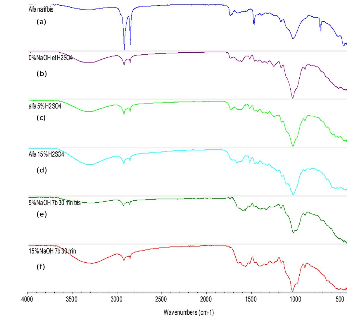
**Figure 7.** FTIR spectra of untreated and pretreated Alfa at different concentrations of  $\text{H}_2\text{SO}_4$  spraying solutions: (a) untreated; (b) pretreated without catalyst; (c and d) pretreated with 5 wt% and 10 wt%  $\text{H}_2\text{SO}_4$ ; (e and f) pretreated with 5 wt% and 10 wt% NaOH.
