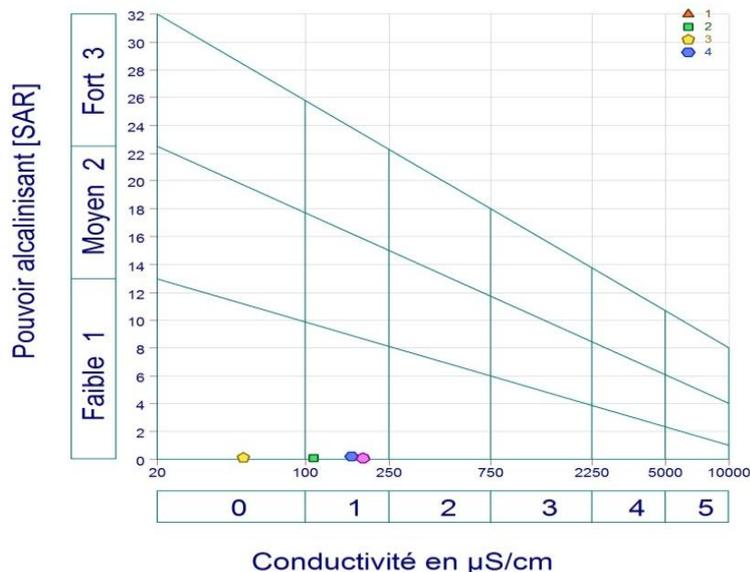
**Figure 3:** Riverside diagram
