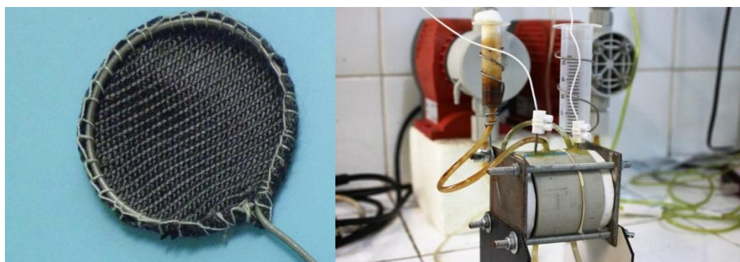
Figure 7: Design of the MFC reactor (A) and the carbon cloth electrodes (B) designed and used in phosphate dissolution experiments.
