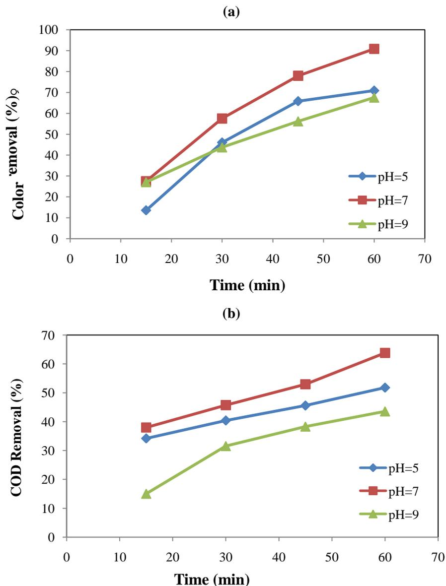
**Fig 2:** Removal efficiency of Al electrode in different pH. a: Color removal, b: COD removal
