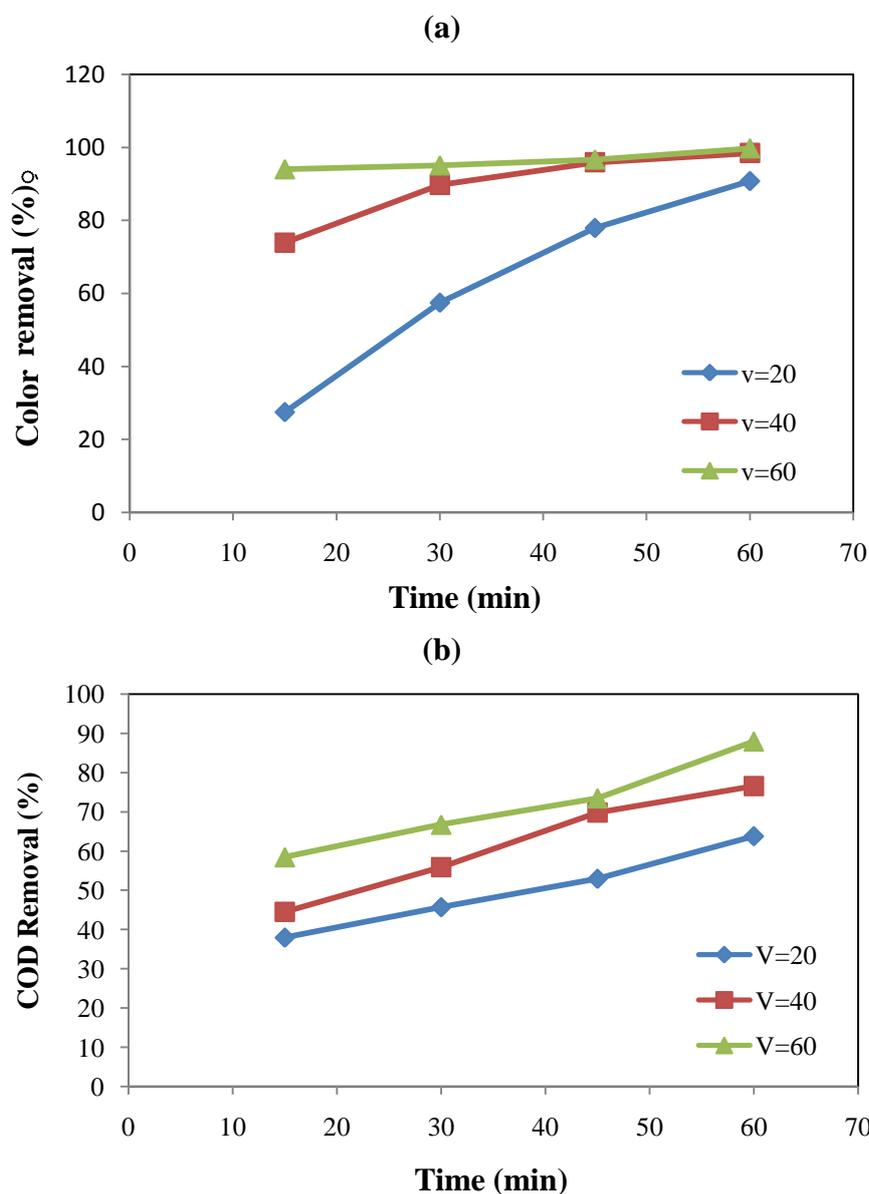
**Fig 4:** Removal efficiency of Al electrode in different voltage and constant pH of 7. a: Color removal b: COD removal.
