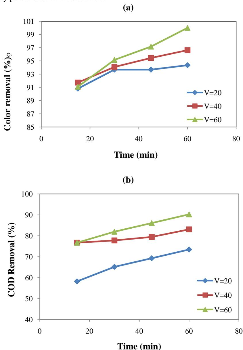
**Fig 3:** Removal efficiency of Fe electrode in different voltage. a: COD removal, b: color removal efficiency.
