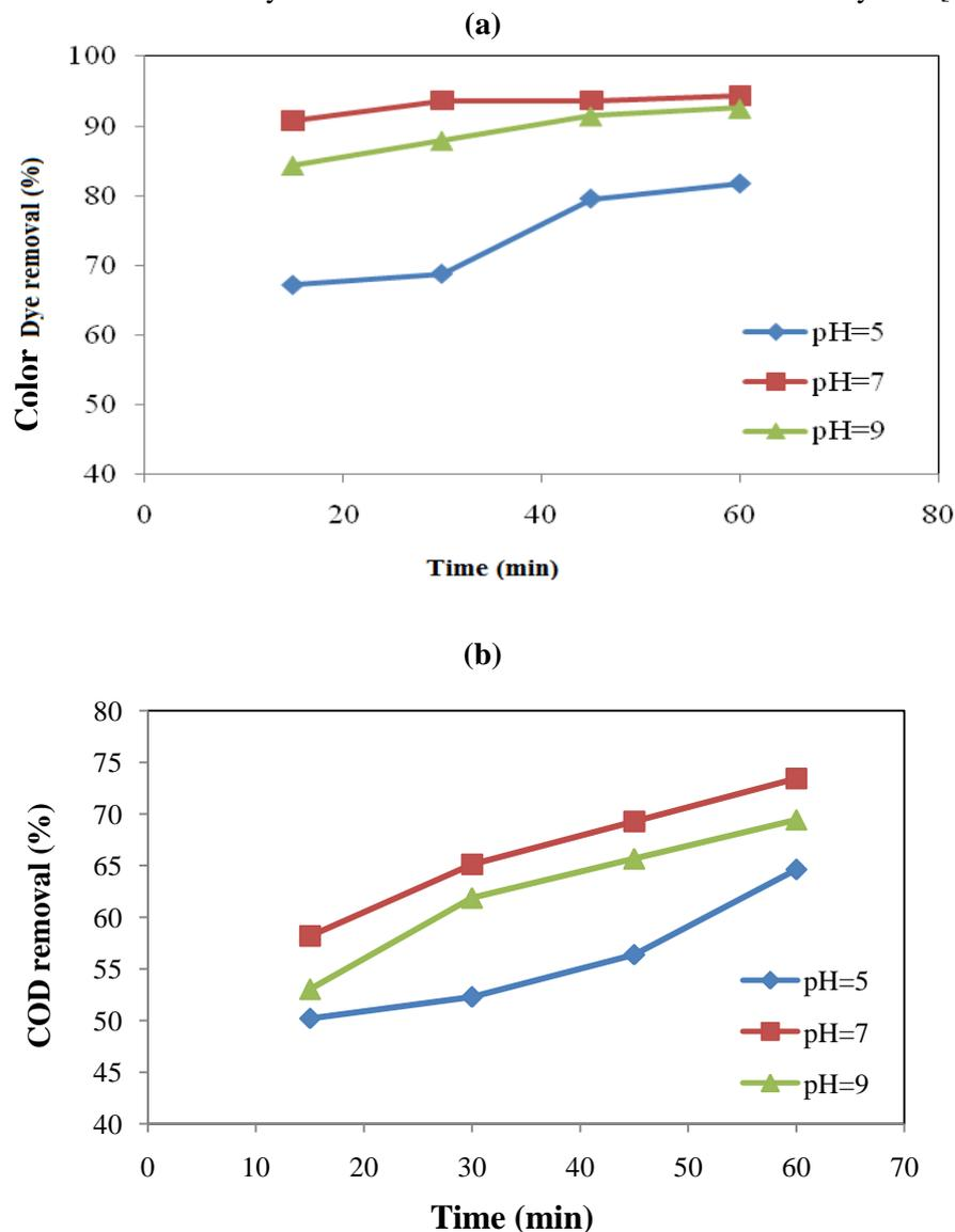
**Fig 1:** Removal efficiency of Fe electrode in different pH. a: Color removal, b: COD removal.
