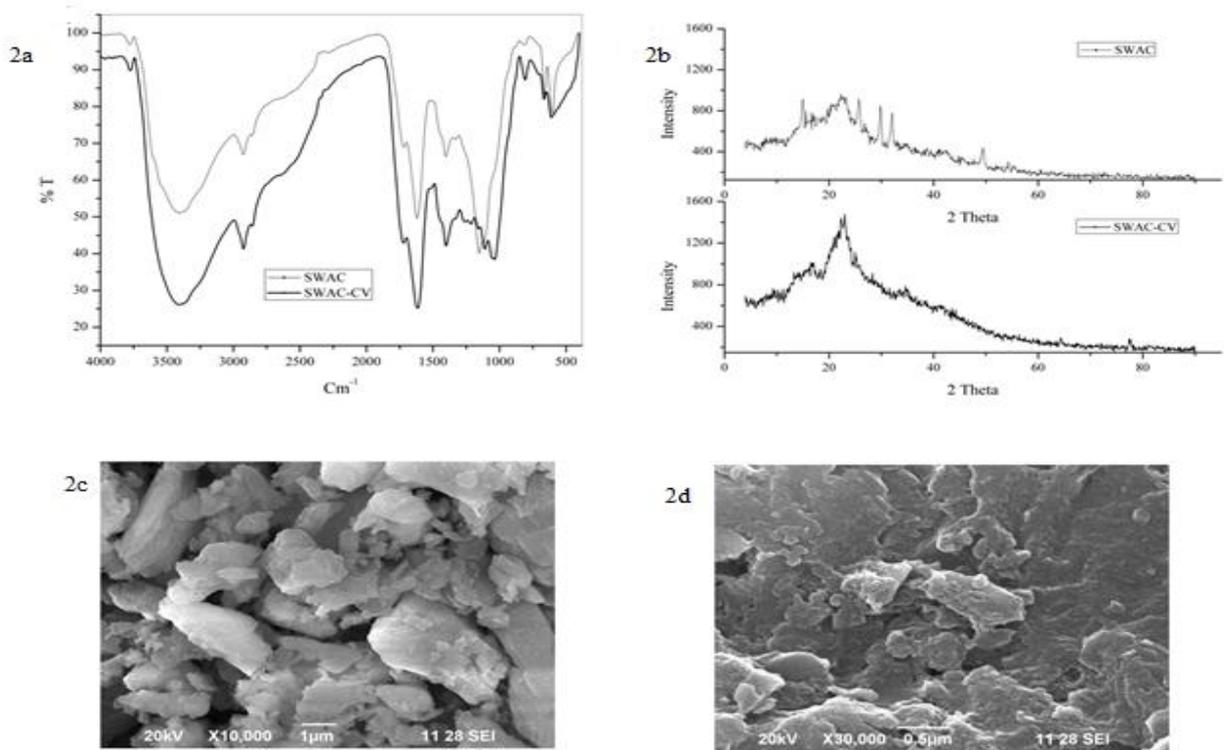
**Figure.2** a)FTIR of SWAC and SWAC-CV dye, **Figure.2 b)** XRD of SWAC and SWAC-CV dye **Figure.2 c)** SEM image of SWAC, **Figure.2 d)** SEM image of SWAC-CV dye
