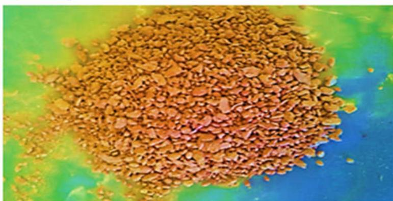
**Figure 1.** SSF/MRR composite blend before pressing.
