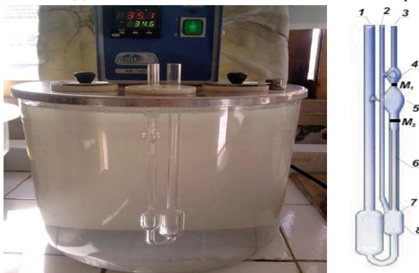
Figure 1: viscosimetric measurement device Ubbelohd VB-1423
