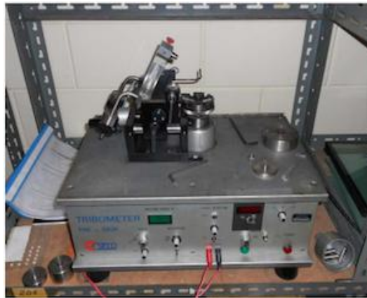
Figure 2: Equipment of pin-on-disc test (CRIBC) [19].
