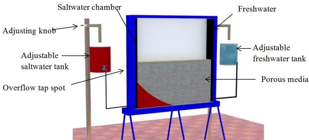
**Figure 1:** Details of the experimental box used in this study
