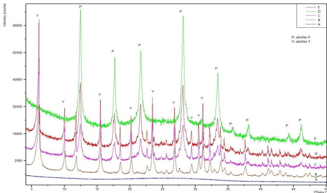
**Figure 5 :** XRD spectrum of samples aged for 24h at room temperature with crystallization at 100°C for 6h (A) 24h (B) 48h (C) 72h (D) and 168h (E)
