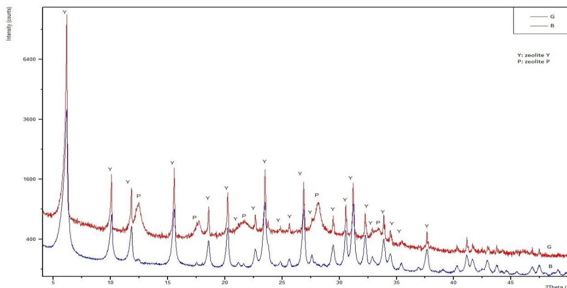
**Figure 1:** XRD spectrum of samples aged for 8(G) and 24h (B) at room temperature
