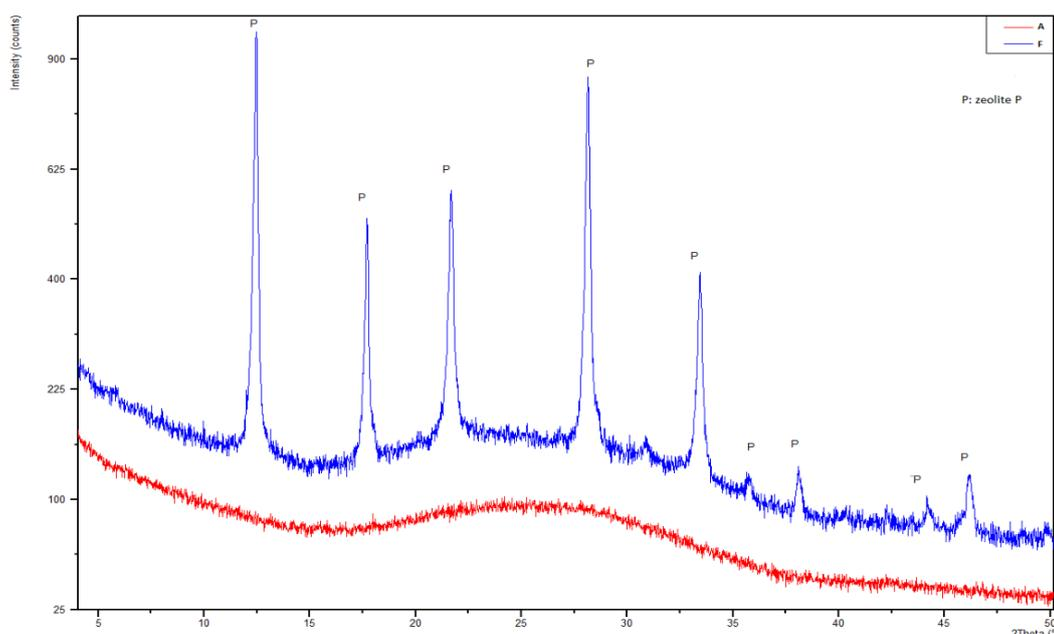
**Figure 3:**XRD spectrum of samples aged for 24h at room temperature (A) and 80°(F) with crystallization for 6h.
