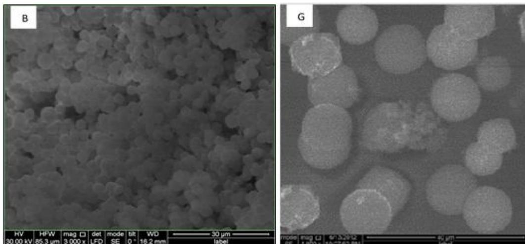
**Figure 2:** ESEM images of samples aged for 8h (G) and 24h (B) at room temperature
