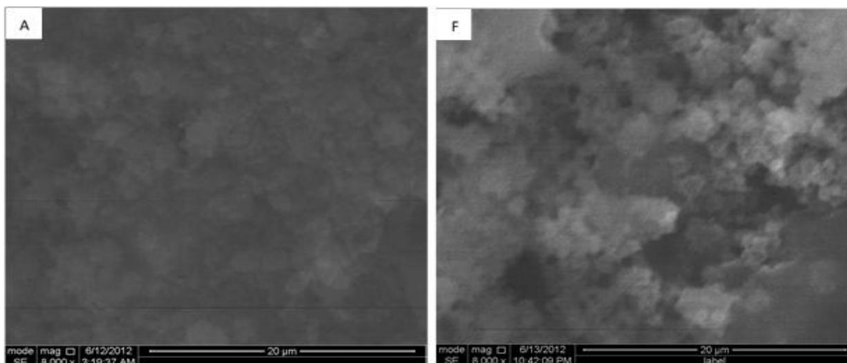
**Figure 4:** ESEM images of samples aged for 24h at room temperature (A) and 80° (F) with crystallization for 6h.
