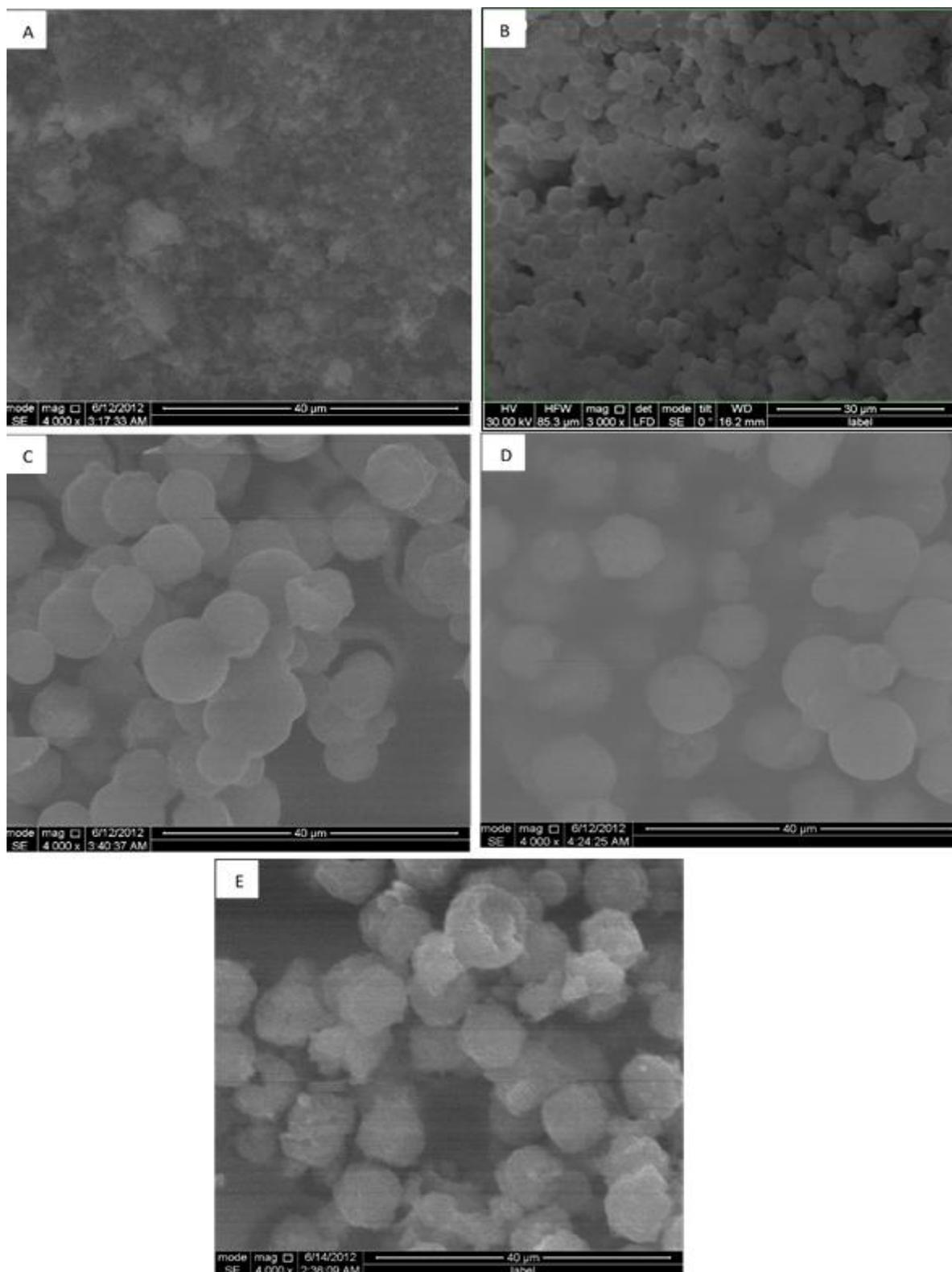
**Figure 6 :**ESEM Images of samples aged for 24h at room temperature with crystallization at 100°C for 6h (A) 24h (B) 48h (C) 72h (D) and 168h (E)
