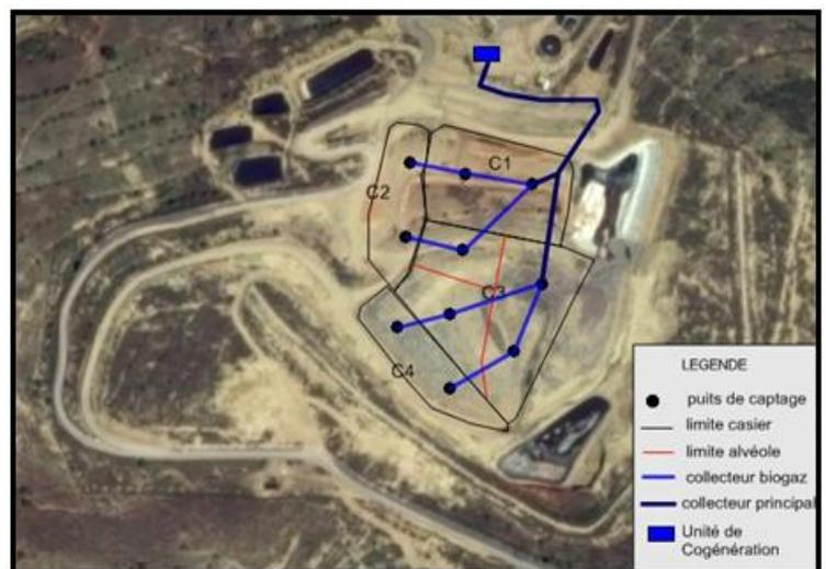
**Figure 7:** Design results for the biogas collection network
